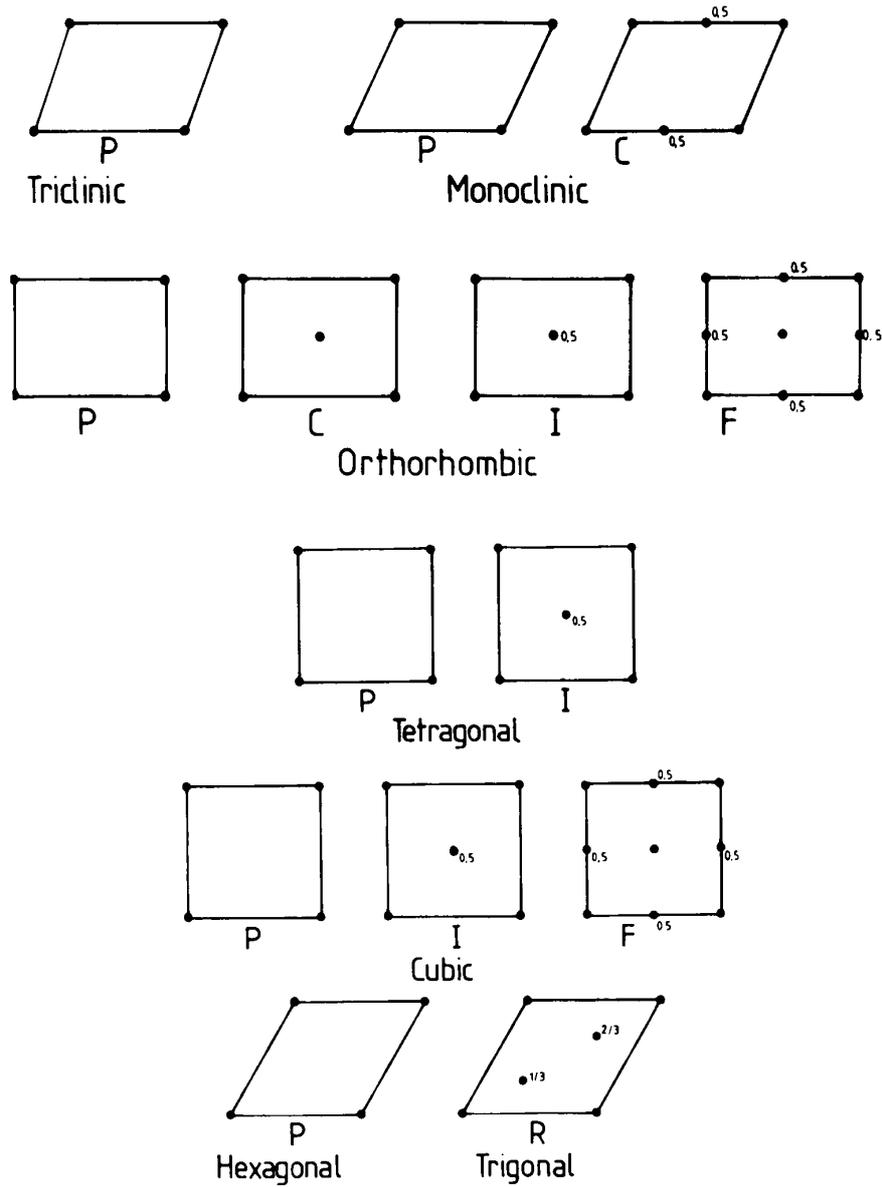
Fig. 1: Projections of the fourteen Bravais lattices along the  $a_3$  axis. The numbers indicate the coordinates of lattice points relative to the  $a_3$  axis; the unlabelled lattice points are by implication located at coordinates 0 and 1 with respect to the  $a_3$  axis. Note that the  $P$ ,  $F$ ,  $I$ ,  $C$  and  $R$  type cells contain 1, 4, 2, 2 and 3 lattice points per cell, respectively.
