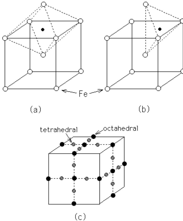
Fig. 11: The main interstices in the body-centred cubic structure of ferrite. (a) An octahedral interstice; (b) a tetrahedral interstice; (c) location of both kinds of interstices.
