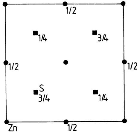
Fig. 8: Projection of the zinc blende crystal structure along the  $a_3$  axis.
