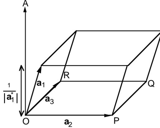
Fig. 3: The relationship between  $\mathbf{a}_1^*$  and  $\mathbf{a}_i$ . The vector  $\mathbf{a}_1^*$  lies along the direction  $\underline{OA}$  and the volume of the parallelepiped formed by the basis vectors  $\mathbf{a}_i$  is given by  $\mathbf{a}_1 \cdot \mathbf{a}_2 \wedge \mathbf{a}_3$ , the area  $OPQR$  being equal to  $|\mathbf{a}_2 \wedge \mathbf{a}_3|$ .
