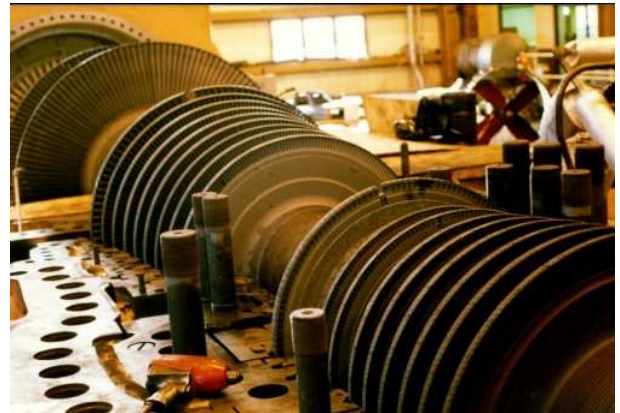
Figure 1.2: Turbine-generator set. In the foreground is the high pressure turbine, follow the intermediate and low pressure turbines, and eventually in background is the generator [1].
