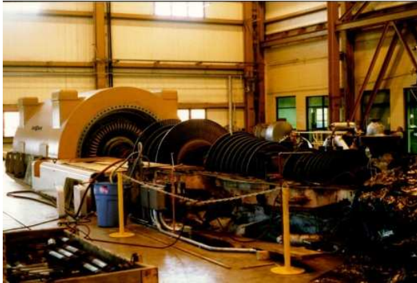
Figure 1.2: Turbine-generator set. In the foreground is the high pressure turbine, follow the intermediate and low pressure turbines, and eventually in background is the generator [1].
