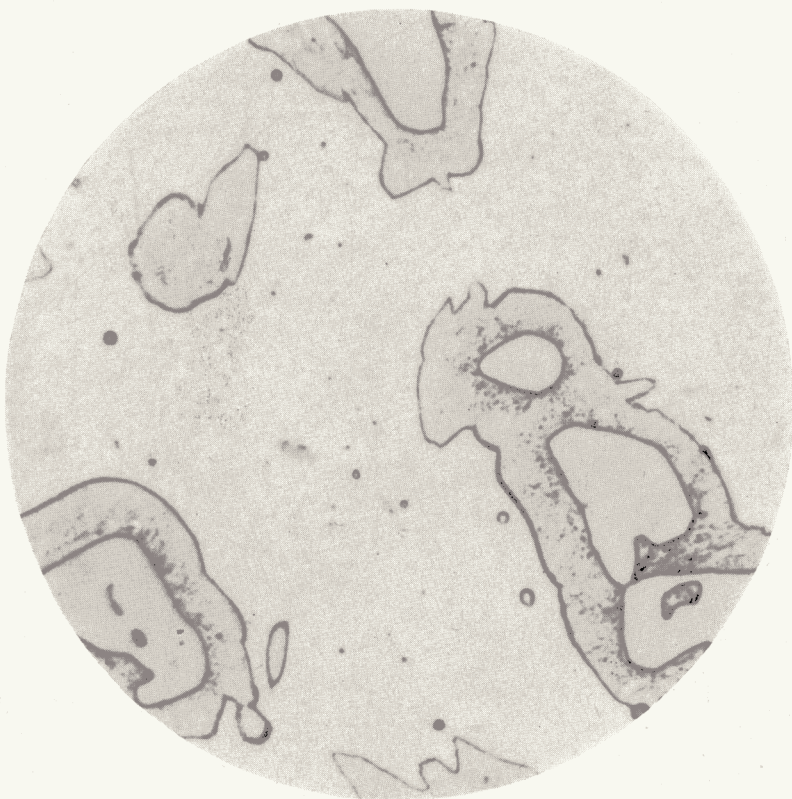
Fig. 59—Photomicrograph of Steel shown in Fig. 58 after Holding about 5 Seconds at 1375 Degrees Fahr. and Quenching. Note Extent of Carbon Diffusion to form Austenite (Now Martensite); (2000 \times ). ( Vilella ).
