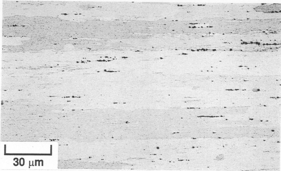
Figure 1.1: Typical microstructure of the mechanically alloyed ODS metal, MA956, after a recrystallization heat-treatment. The extrusion is horizontal in this micrograph.
