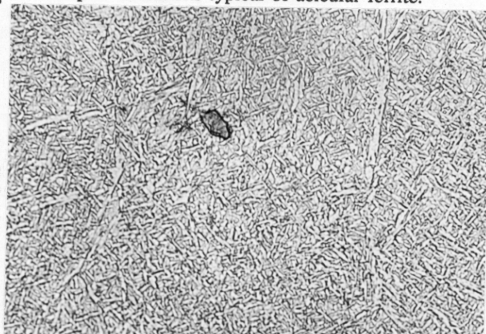
Figure 4.1. 0.7 \mu m Star shaped formations typical of acicular ferrite.
