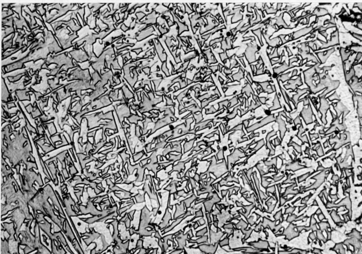
Figure 4.1. 0.7 \mu m Star shaped formations typical of acicular ferrite.
