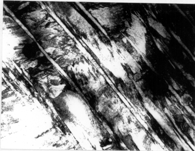
Figure 5.17. Retained \gamma rimming bainite laths. PJ306, 1000°C/10 mins-680°C/1800s.
