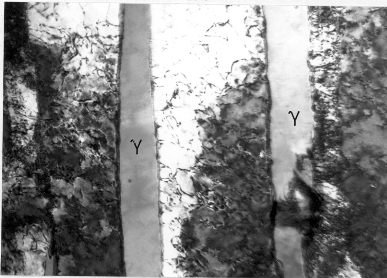
Figure 5.26. Retained \gamma between Widmanstätten \alpha plates. PJ305, 1000°C/10 mins-500°C/317s.
