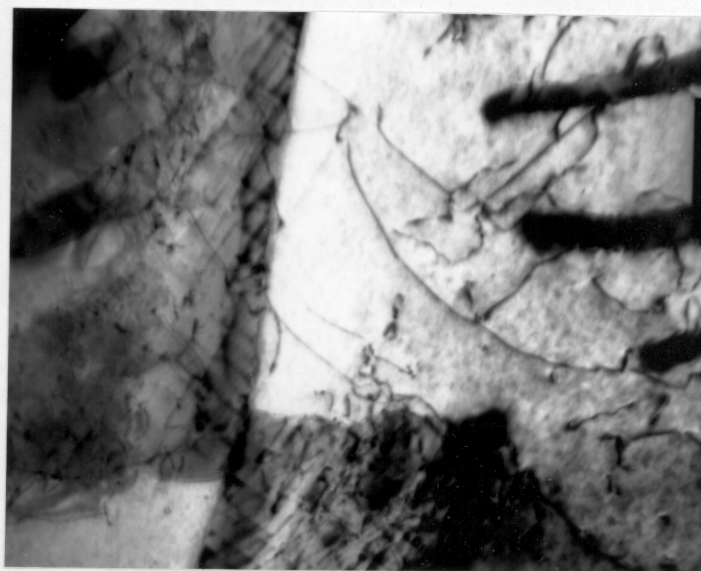
Figure 5.23. Dislocation cells in fully pearlitic microphase. PJ306, 1000°C/10 mins-680°C/73800s.
