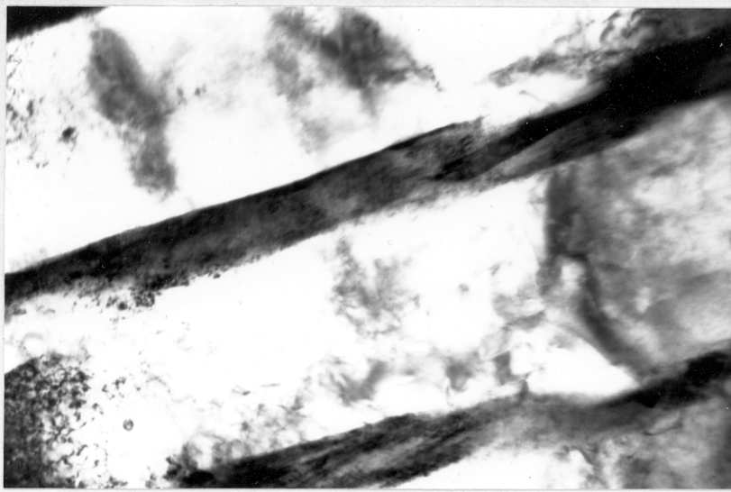
Figure 5.24. Twinned martensite between Widmanstätten \alpha plates. PJ305, 1000°C/10 mins-500°C/80s.
