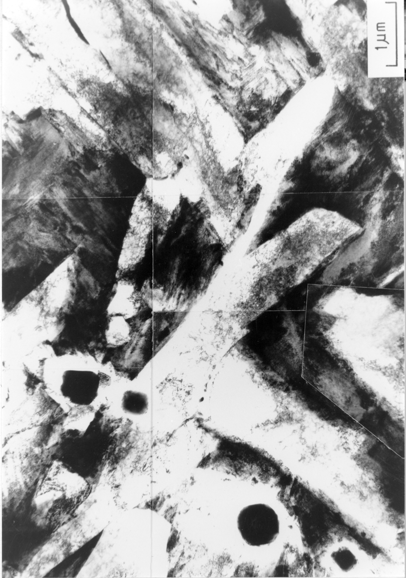
Fig. III.7b - Transmission electron micrograph shows acicular ferrite. Weld metal was reaustenitised at 1200°C for 30 minutes, followed by isothermal transformation at 460°C for 30 minutes and then quenched by helium jets.
