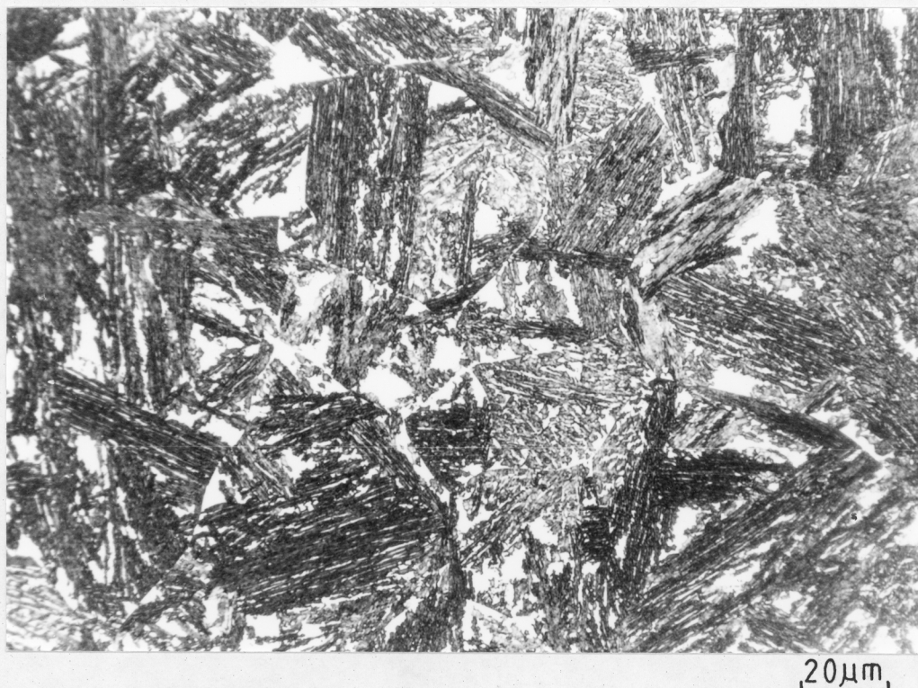
Figure VII.2 - Optical micrograph showing the upper bainitic ferrite and residual austenite (blocky and film morphologies) following isothermal transformation at 350°C for 120 minutes.
