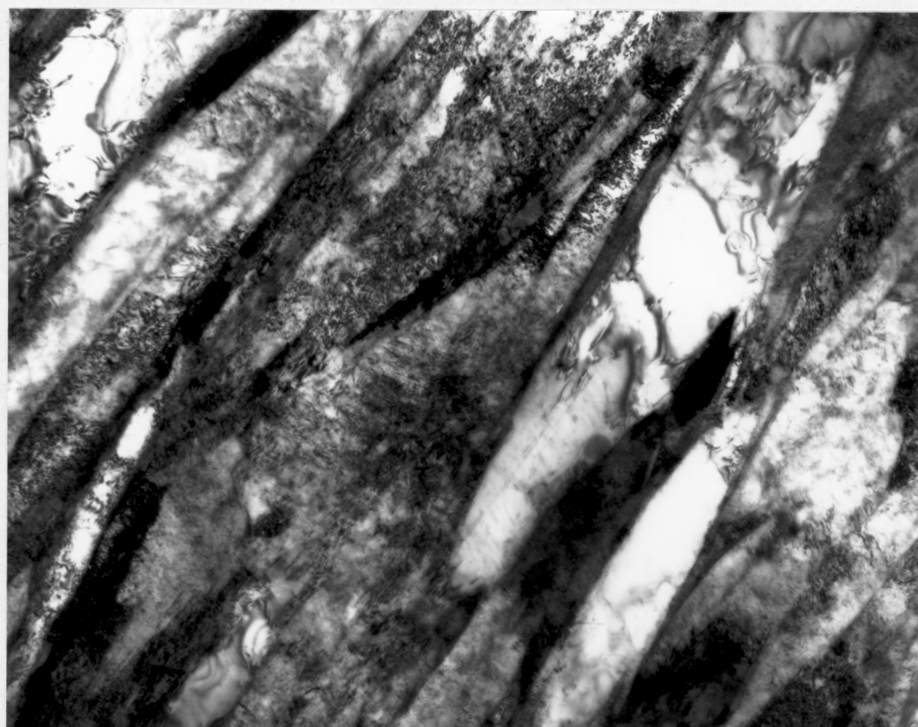
Figure VII.14e - 10 mins @ 950°C → 2 hrs @ 350°C → 2 hrs @ 780°C → quenched by helium gas.
