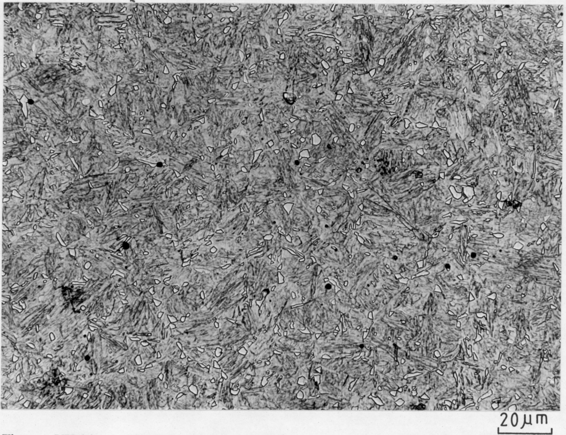
Figure VII.14g - Optical micrograph showing the microstructure after isothermal reaustenitisation at 820°C for 2 hrs. (10 mins @ 950°C → 2 hrs @ 350°C → 2 hrs @ 820°C → quenched by helium gas).
