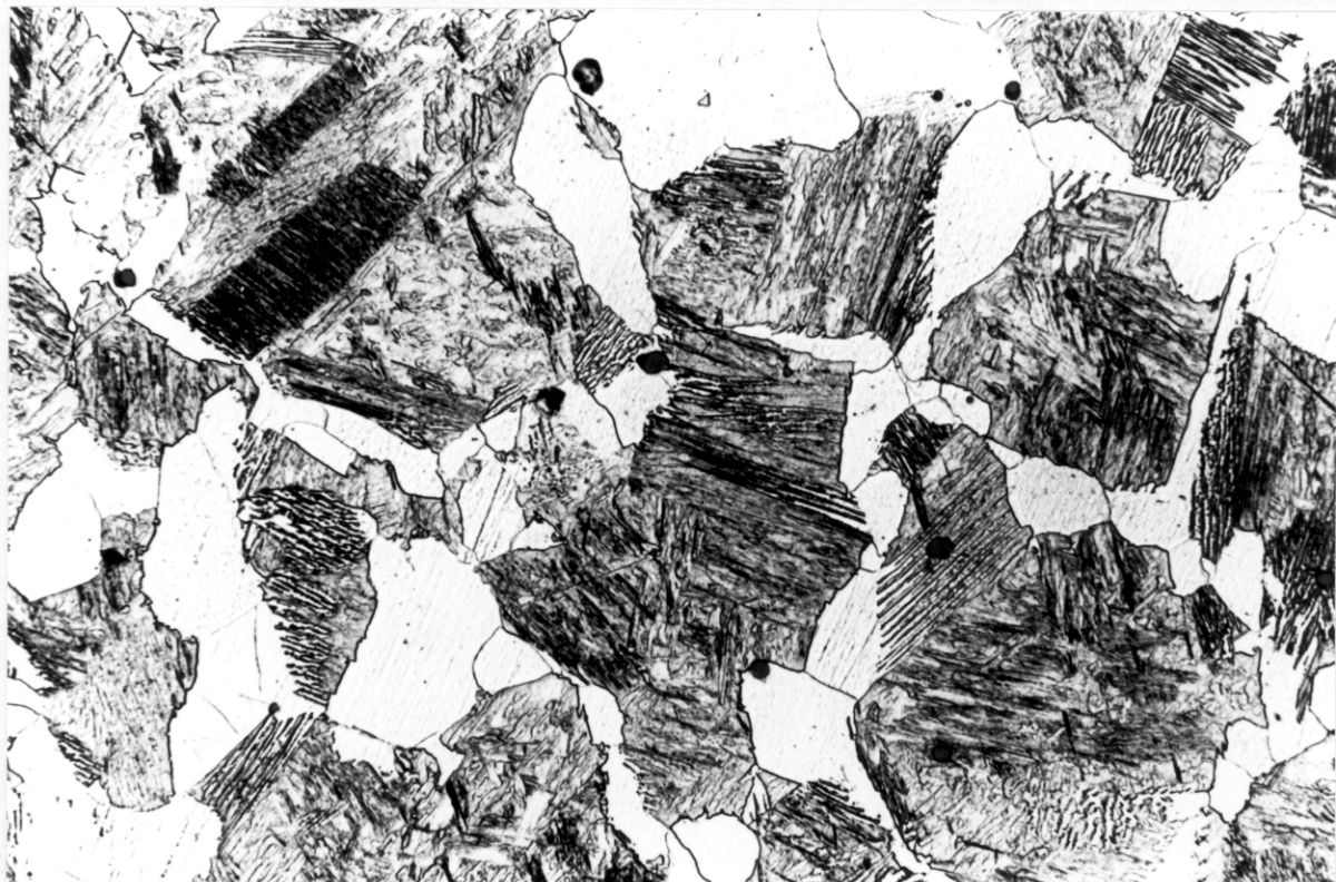
Figure VIII.8(f)-10 mins @ 1100°C → 2 hrs @ 700°C → quenched by helium gas. 20μm
