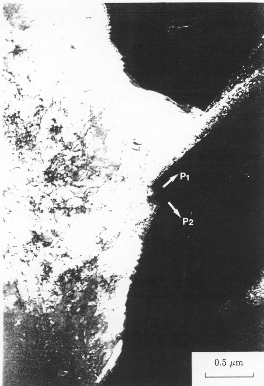
Fig. 7.9 The micrograph of the interface which showed KS/NW relation with the austenite, exhibiting ledge type faceted interface. The ledge height can be seen to vary over the width of the ferrite, apparently increasing towards the nucleation site of bainite.
