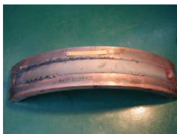
A 120 degree weld segment
