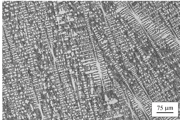
Figure 5.4(e): - A typical micrograph from the test plate for condition 3 in Table 5.1. This overlay was hypoeutectic. Dendrites of austenite can be seen in the structure. The dendrites are surrounded by the eutectic constituent.
