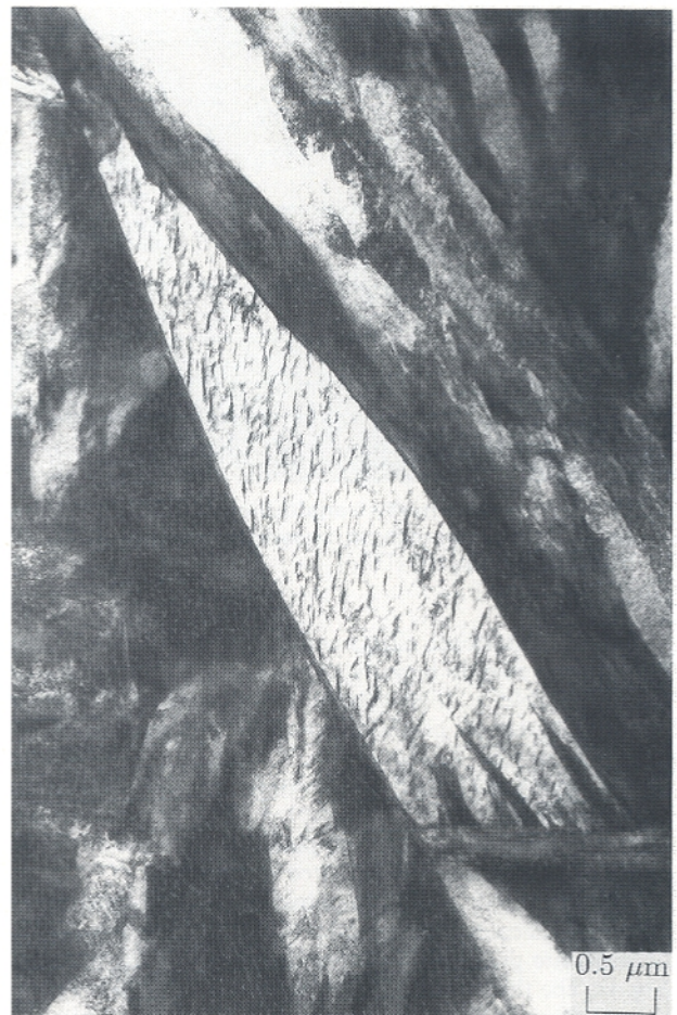
3 Alloy H1, isothermally transformed at 305°C for 150 s before quenching in thermomechanical simulator showing coalescence and intense carbide precipitation in all parts of bainite, i.e. subunits before and after coalescence (TEM)
