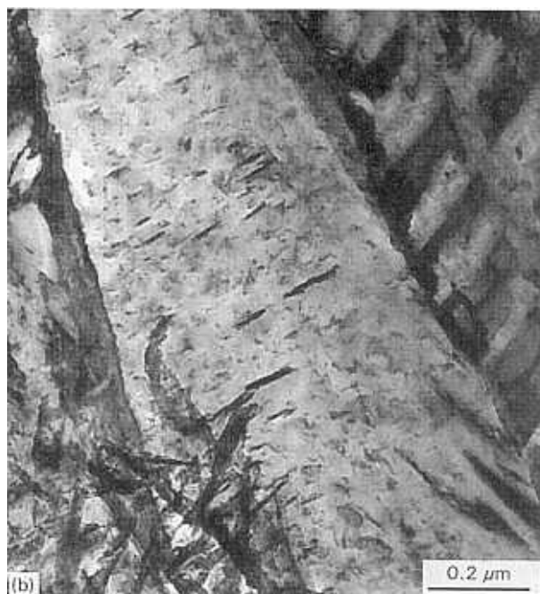
Figure 4 Two examples of lower bainite that has formed under the influence of a compressive stress of 700 MPa. Both cases show a clear tendency for the carbides to precipitate in a single orientation. These micrographs should be compared with Fig. 3b.
