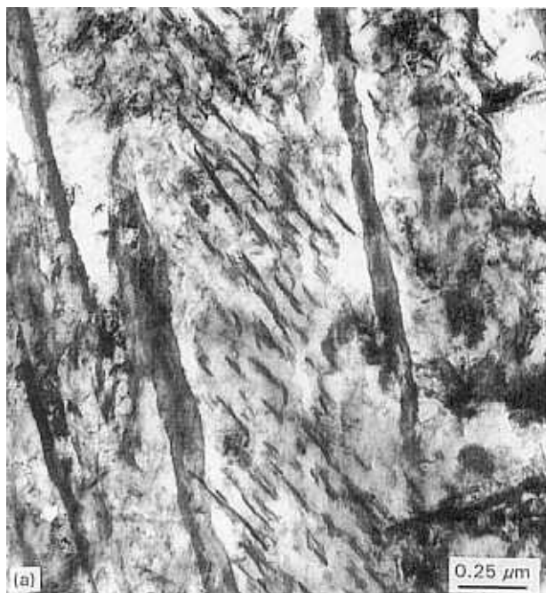
Figure 4 Two examples of lower bainite that has formed under the influence of a compressive stress of 700 MPa. Both cases show a clear tendency for the carbides to precipitate in a single orientation. These micrographs should be compared with Fig. 3b.
