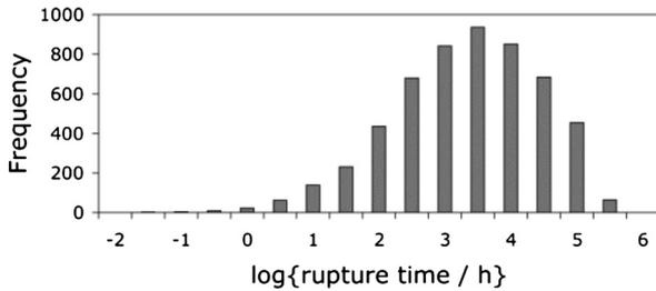
**Fig. 1.** The distribution of creep rupture times in the dataset used to create the published model for the estimation of the creep strength of ferritic steel plates.
