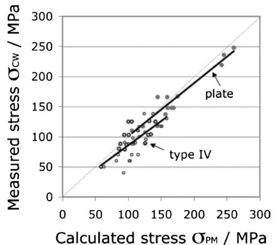
**Fig. 2.** Measured cross-weld rupture strength versus that calculated using the plate neural network model. The solid points correspond to failure either in the base metal or weld metal, whereas the open points correspond to tests that resulted in Type IV failure.
