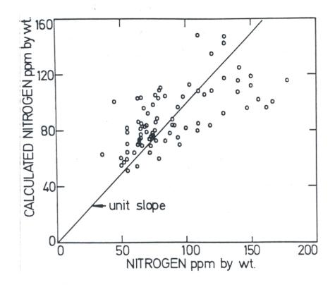
[1] Comparison of calculated (eq.6) and actual nitrogen concentrations of manual metal arc welds.
