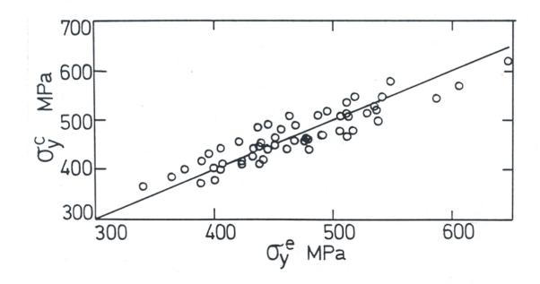
[2] Comparison of calculated and actual yield strengths of multirun manual metal arc weld deposits.
