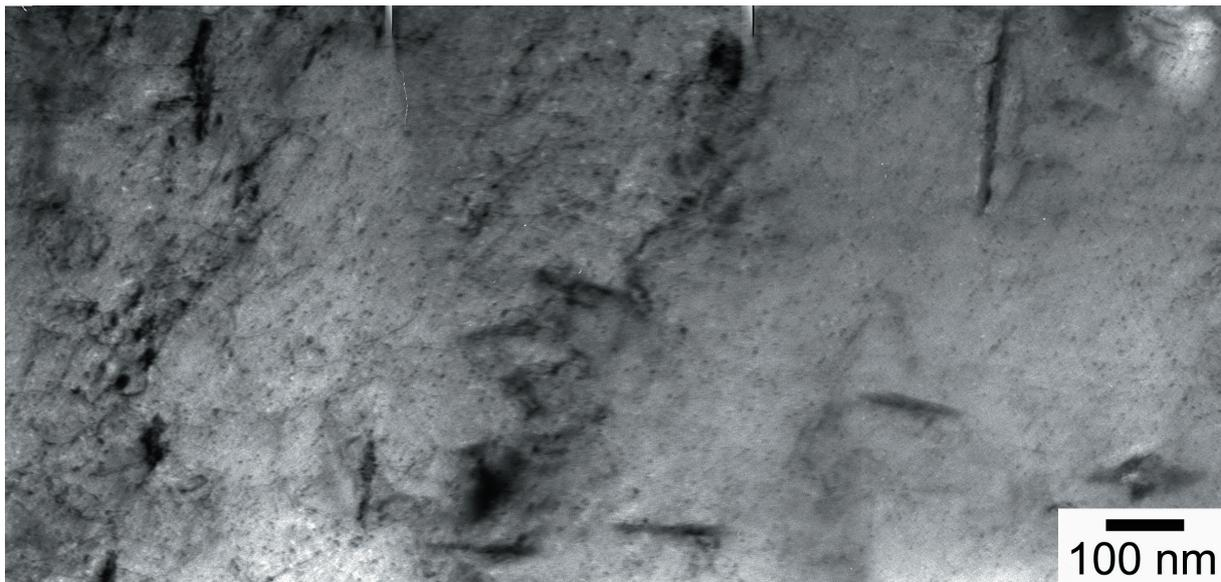
**Figure 6** Higher magnification bright field TEM micrograph showing the precipitates within the same grain as in Figure 5.
