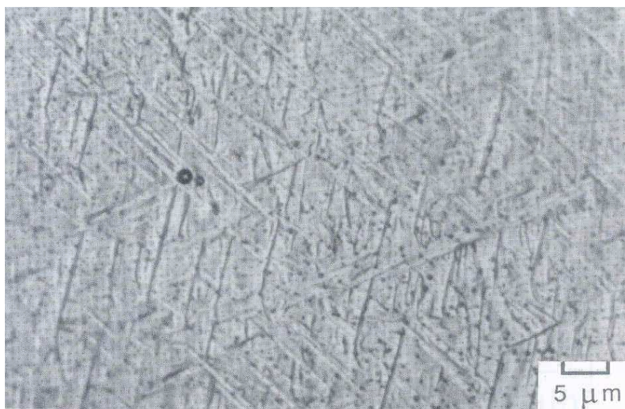
Fig. 14: Nomarski interference contrast micrograph from a surface relief experiment in which a sample was metallographically polished and then transformed to acicular ferrite in an inert protective atmosphere (Strangwood and Bhadeshia, 1987).
