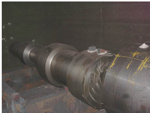
Fig. 10 Trial rotor forgings
