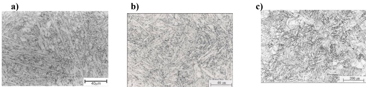
Fig.5 Comparison of the optical micrographs after oil quenching and double tempering. a) Alloy A b) Alloy B c) Alloy C
