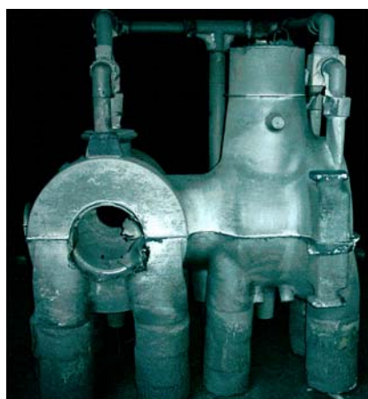
Fig. 12. 617 valve chest casting after removal from mould and shot peening (courtesy of Goodwin Steel Castings)
