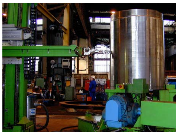
Fig. 13. 617 forging during automatic ultrasonic inspection (courtesy of Saarschmiede)
