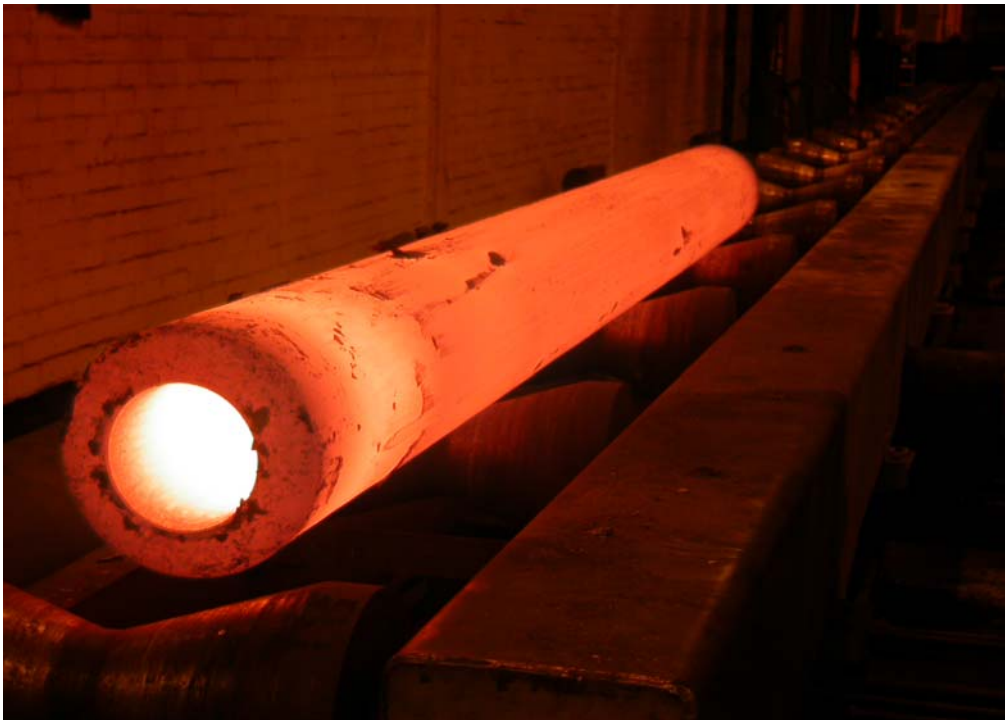
Fig. 7. Extruded NIMONIC ® alloy 263 steam pipe
