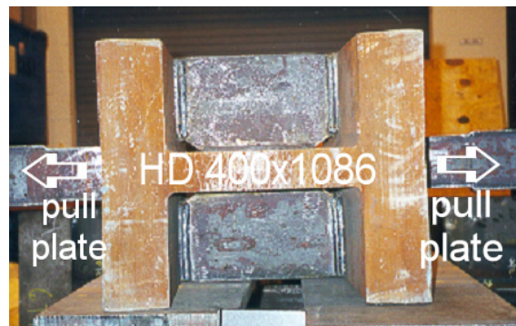
Fig. 6: Through-thickness tension test on ‘jumbo’ column HD 400x1086 in HISTAR 460
