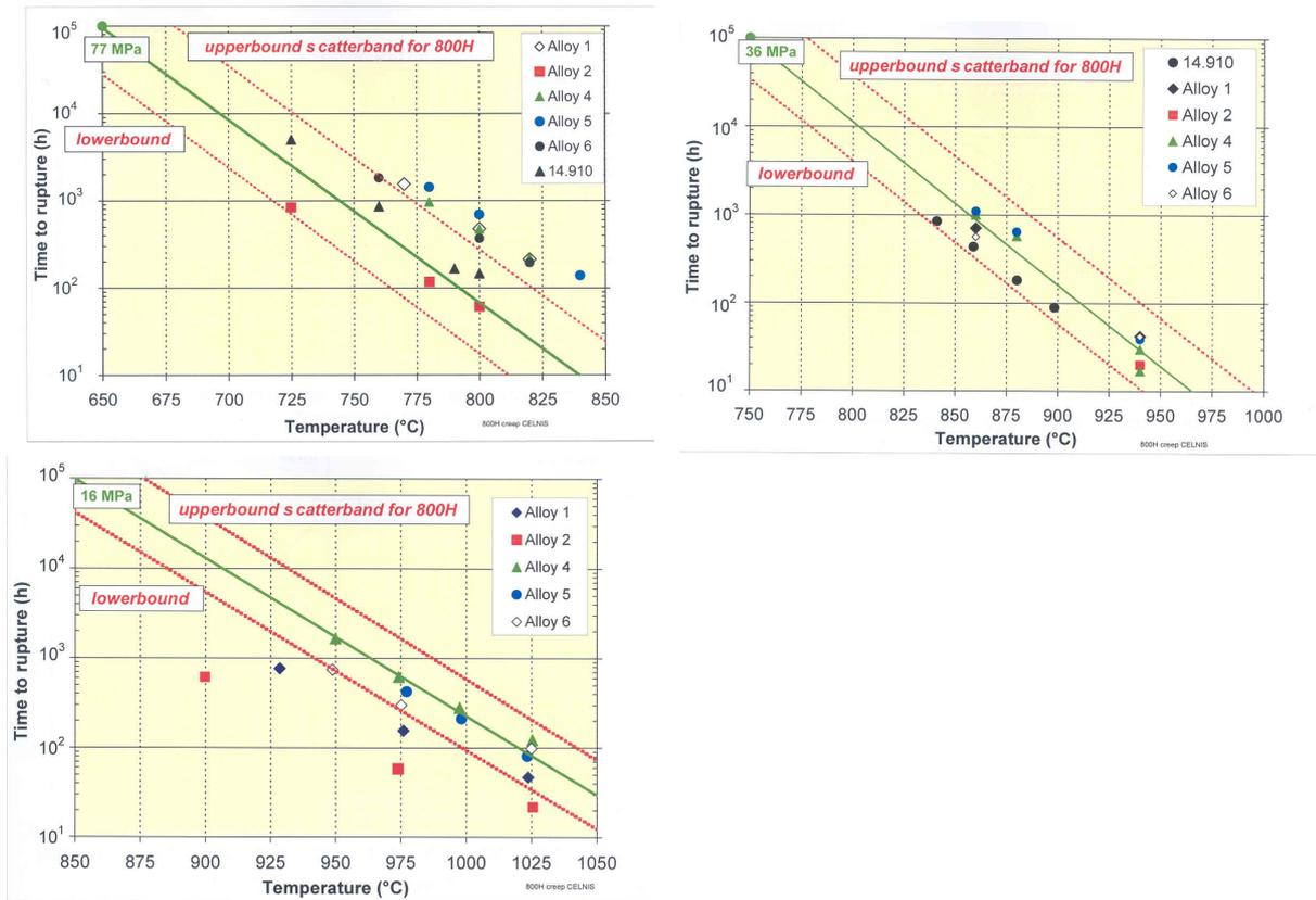
Fig. 7: Results of isostress creep tests with stress level of 77MPa, 36MPa and 16MPa
