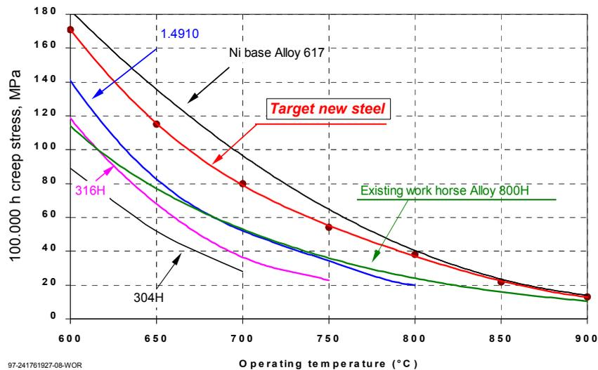
Fig. 1:  $10^5$ h creep rupture strength new austenitic steel (target) compared to existing materials.
