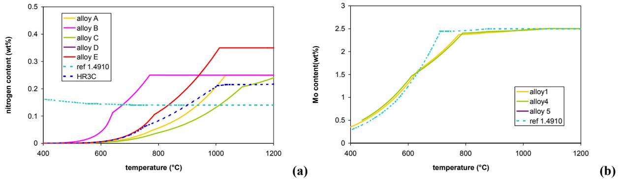
**Fig. 4: Calculated equilibrium nitrogen (a) and molybdenum (b) content in the austenitic matrix phases as function of temperature**
