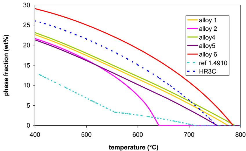
**Fig. 3: Calculated equilibrium fraction of intermetallics phases as function of temperature**
