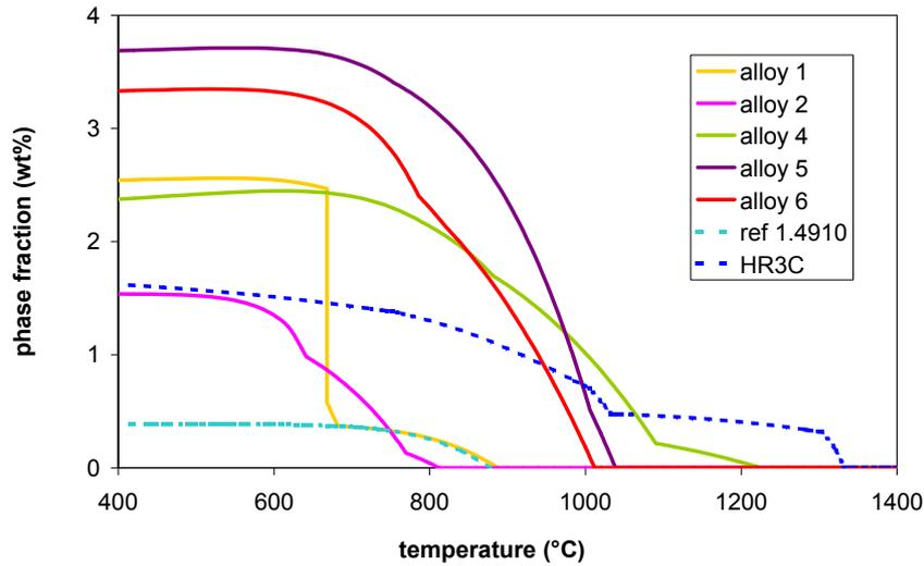
**Fig. 2: Calculated equilibrium fraction of carbides and carbonitrides as function of temperature**
