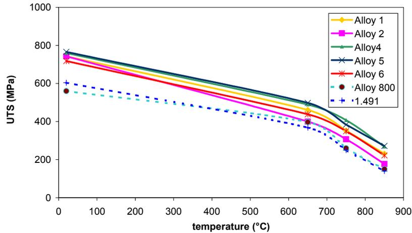
Fig. 5: Tensile strength of 5 laboratory heats and 2 reference materials
