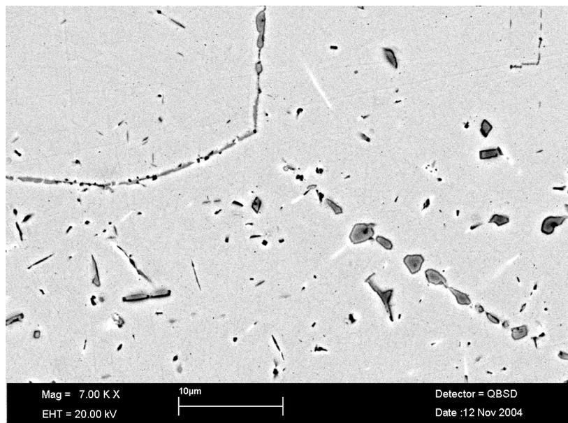
**Fig. 8: Second phase distribution on the grain boundary and inside the grains of the alloy 4**
