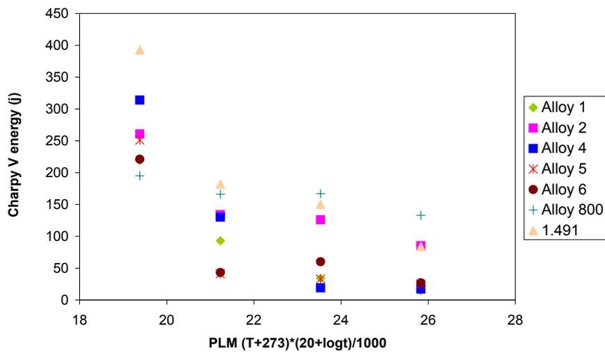
Fig. 6: Toughness of 5 laboratory heats and 2 reference materials
