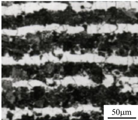
**Figure 5** Banded microstructure in 42CrMo obtained by conventional annealing (the rolling direction is horizontal in the picture) [29].
