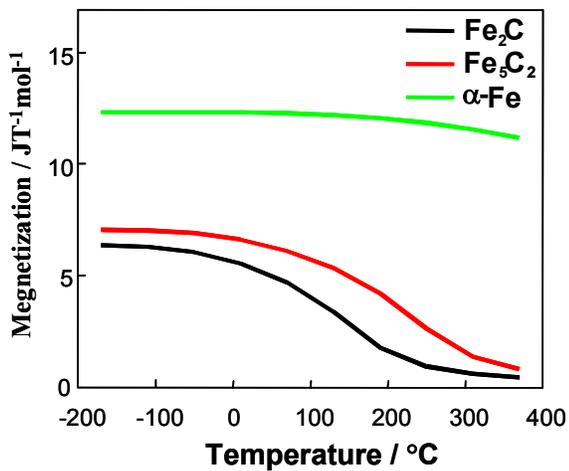
**Figure 11** Temperature variations of magnetization of Fe<sub>2</sub>C, Fe<sub>5</sub>C<sub>2</sub> and α-Fe [35].
