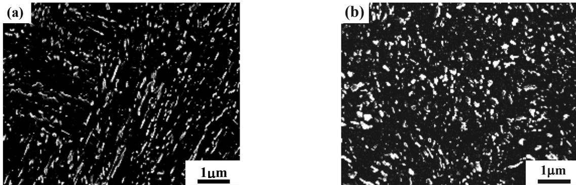
**Figure. 7** SEM micrographs of carbide obtained by being tempered at 650°C for 1 h (a) without magnetic field; (b) with a 14-T magnetic field. The field direction is vertical. SEM secondary electron images [34]
