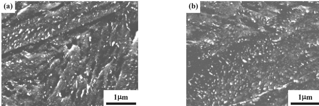
**Figure 10** SEM secondary electron images of carbide precipitates (bright areas) within martensite in specimens tempered at 200°C for 60 min (a) without and (b) with a 14-T magnetic field (the magnetic field direction is vertical in the micrograph) [35].
