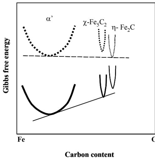
**Figure 12** Schematic diagram of Gibbs free energy vs. carbon concentration for  $\alpha'$  martensite,  $\chi$ -Fe<sub>5</sub>C<sub>2</sub> and  $\eta$ -Fe<sub>2</sub>C at 200°C without (dash line) and with (solid line) a 14-T magnetic field [35].
