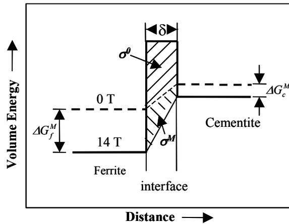
**Figure 8** Schematic illustration of cementite/ferrite interfacial energy without and with the magnetic field
