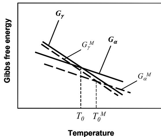
**Figure 1** Variation of Gibbs free energy of austenite and martensite versus temperature in the case without and with magnetic field,  $\alpha$  – martensite ;  $\gamma$  – austenite ;  $M$  – magnetic field
