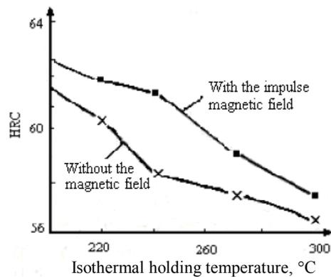
Fig. 3 Hardness of 9SiCr as a function of isothermal holding temperature [21].
