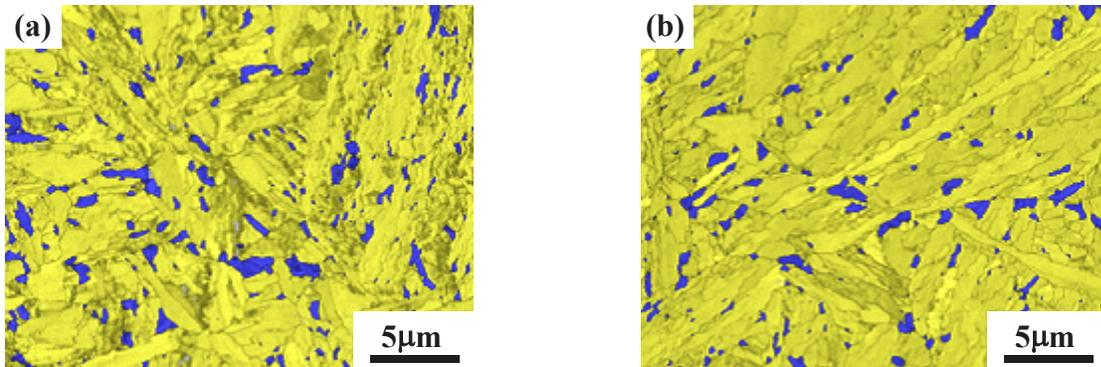
**Figure 9** OIM maps of specimens tempered at 650 for 1 h (a) without field and (b) with a 14-T magnetic field. The field direction is horizontal in the picture [34].
