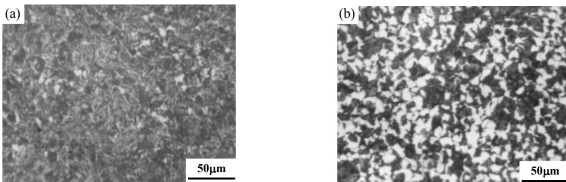
**Figure 4** Microstructure of specimen heat treated at 880°C for 33min and cooled at 46°C/min without (a) and with (b) a 14-T magnetic field, Field direction is vertical in the picture [32]
