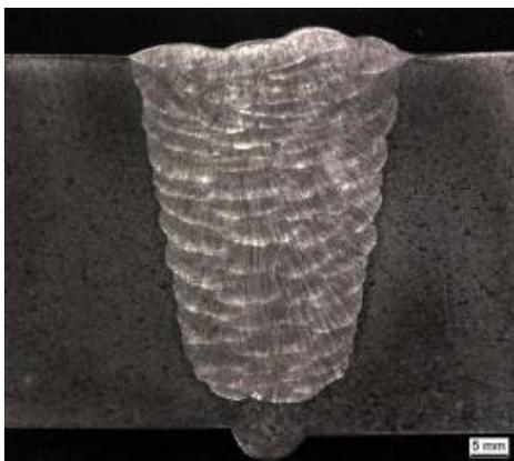
Pipe OD 400 x 50 mm – Butt weld GTAW/SMAW
