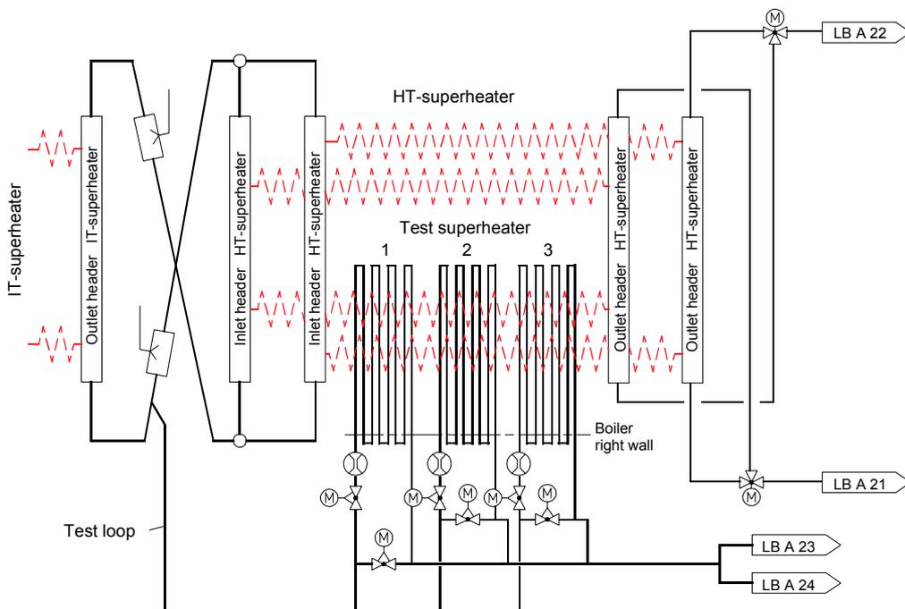
Fig. 3: Esbjerg Test Rig for investigations of advanced materials
