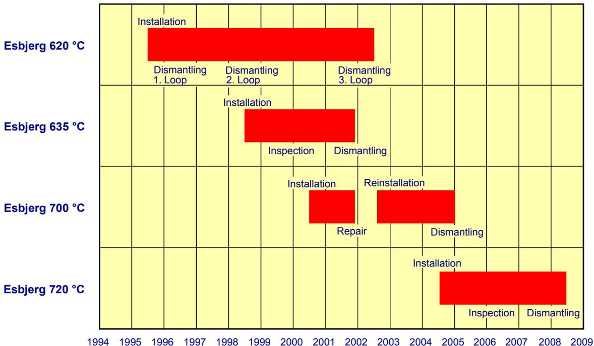
Fig. 5: Test superheaters installed in Esbjerg Test Rig
