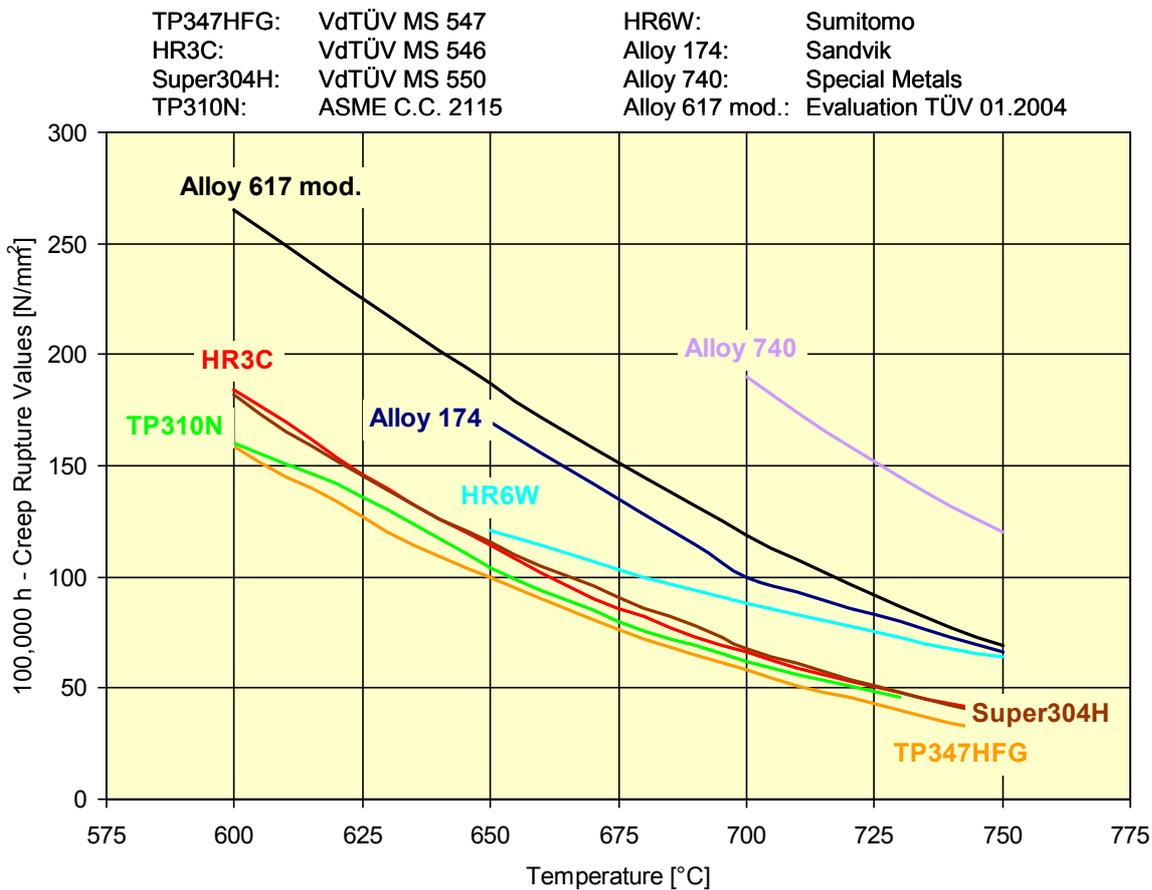
Fig. 7: 100,000 h - creep rupture values of selected materials
