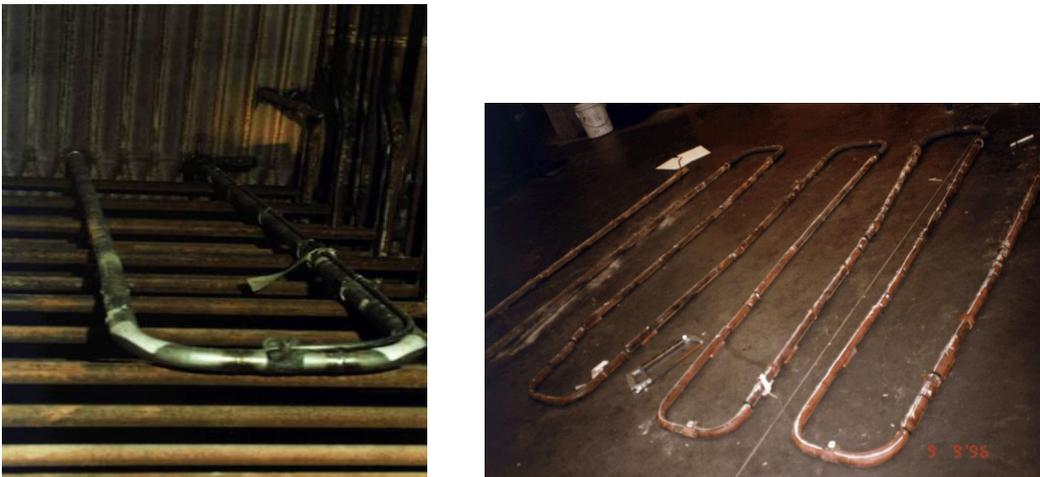
Fig. 4: Test superheaters before and after dismantling
