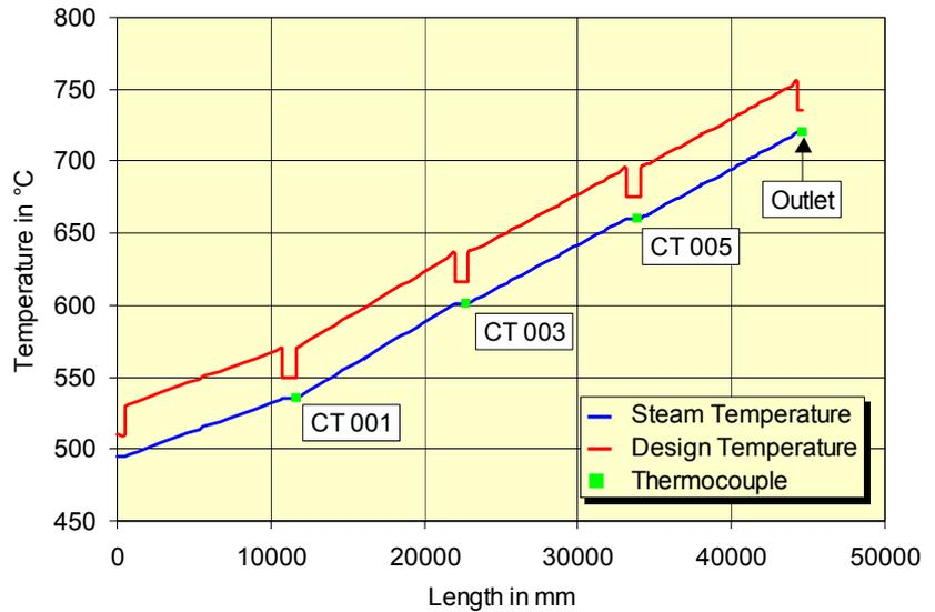
Fig. 9: Temperature profile of the test superheater
