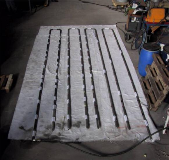
Fig. 14: Test superheater after fabrication
