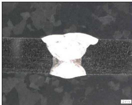
Tube OD 38 x 6.3 mm – Butt weld GTAW
