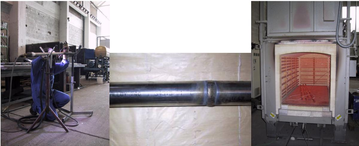
Welding in fixed position      Dissimilar weld      Alloy 740 - heat treatment
