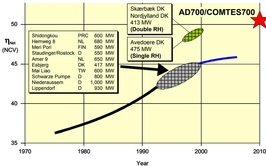
Fig. 1: Development of the power plant efficiency
