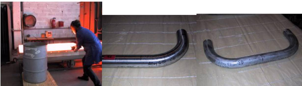
Alloy 617 mod. - heat treatment      Alloy 617 mod. - cold bended      Alloy 174 - cold bended
