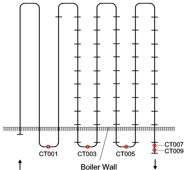
Fig. 8: Design of the test superheater
