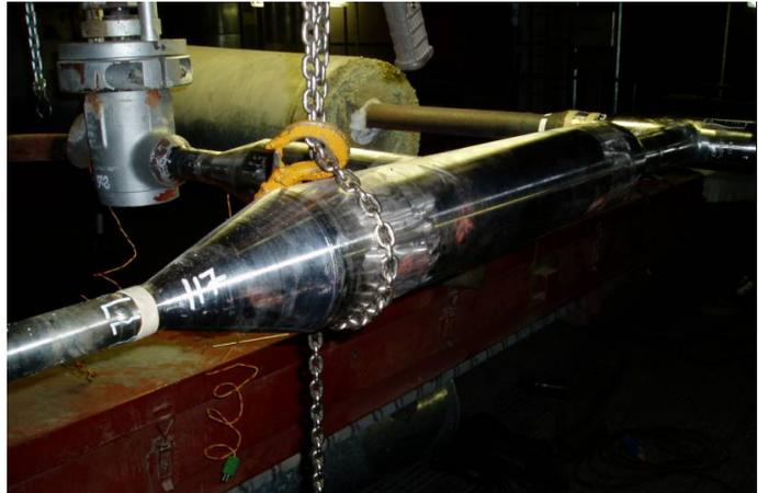
Fig. 15: Mixing piece after erection in the test rig
