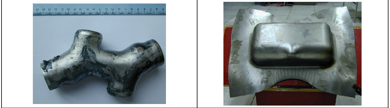
Fig. 2 – Hydroformed parts: an exhaust component and a 304 stainless truck oil sump.
