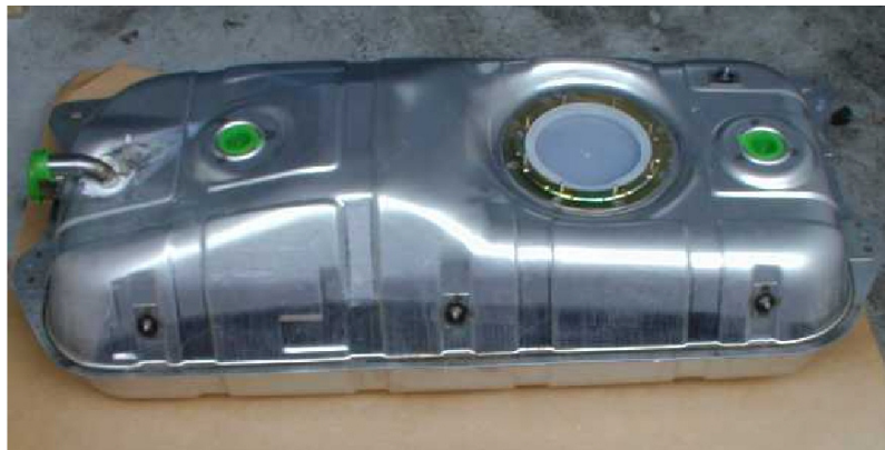
Fig.4 – Fiat Barchetta stainless steel fuel tank, 14301, 0.6 mm thick.
