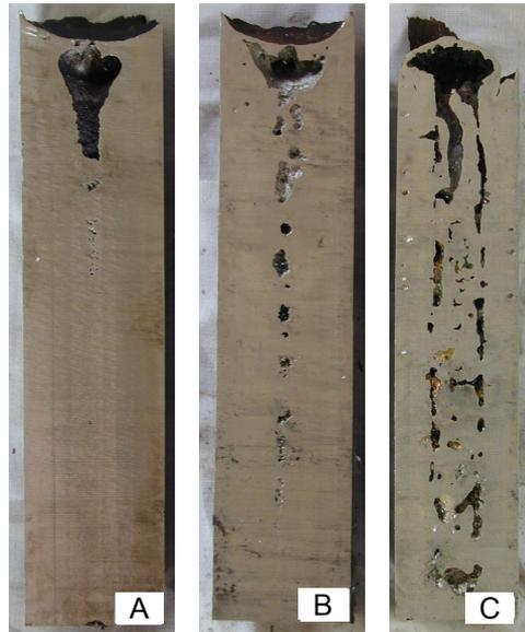
Fig.3. Macrostructure of ingots produced by HF at 0.9 bar
