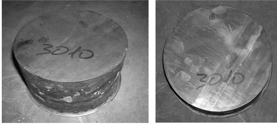
Fig.5. Transversal section of the ingot “E” produced by PESR process at 70 bar
