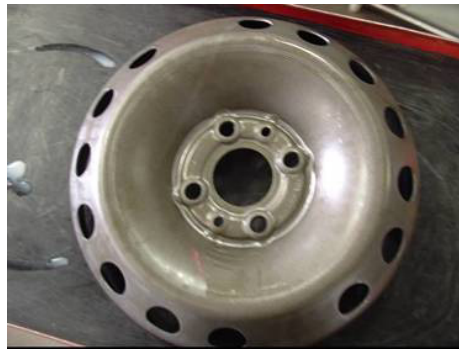
Fig. 8 Disc for wheel made with 3.0 mm thick DP600 strip produced by I.S.P. process.
