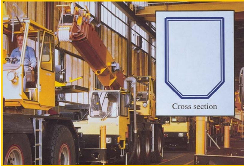
Fig. 4: Design of compression flange for increased buckling load in extra high-strength steel
