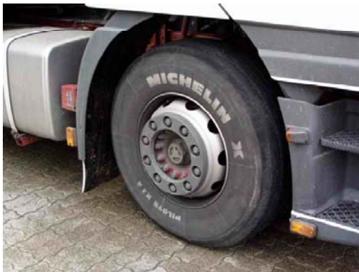
a. Welded steel wheel (22.5 x 9.00)
