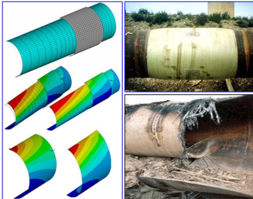
Figure 6 – Crack arrestor modelling and actual test results on X100 pipes [25]
