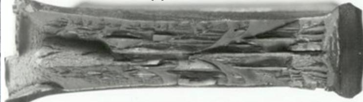
Figure 3 – Comparison between DWTT and WJ test results for an X100 pipe [14]
