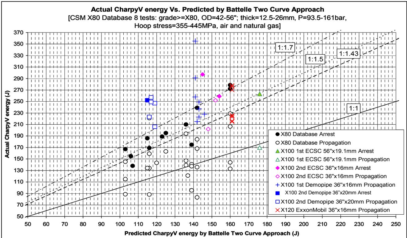
Figure 5 – Actual vs. Predicted CharpyV energy by Battelle Two Curve Approach for high-grade steel linepipes (CSM’s database)
