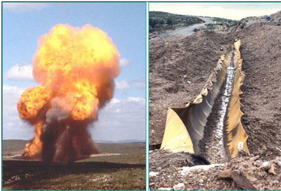
Figure 4 – CSM’s burst test on X100 pipes [23]
