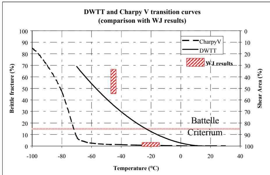
Figure 2 – Comparison between CharpyV, DWTT and WJ test results for an X100 pipe [14]
