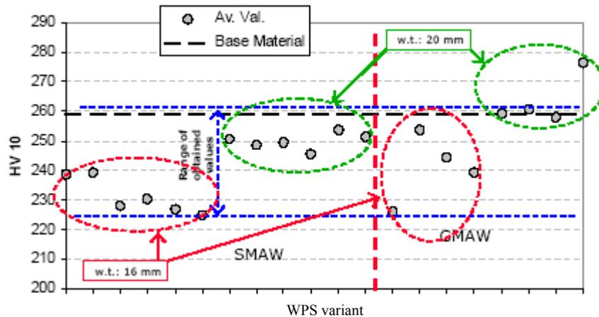
Figure 2: Coarse grained HAZ hardness summary for the various procedure trials
