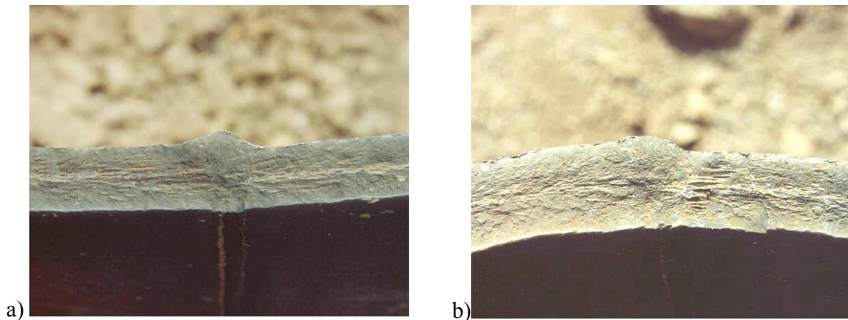
Figure 3: Fracture surface appearance of a) GMAW and b) SMAW joint after burst test.
