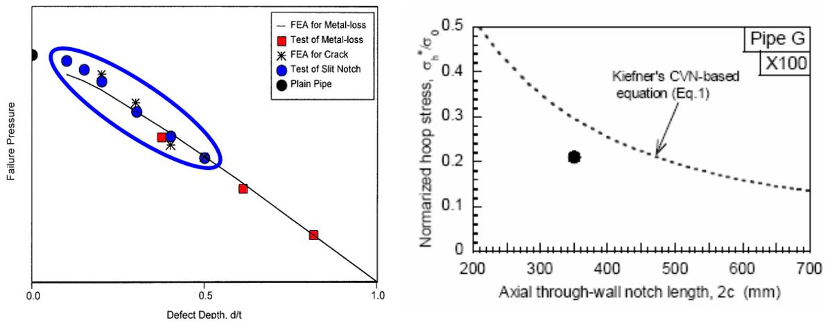
Figure 5: Parent metal axial crack tolerance results for X100 materials. Left, data from [8] for surface breaking cracks; right data from [14] for a through-wall crack
