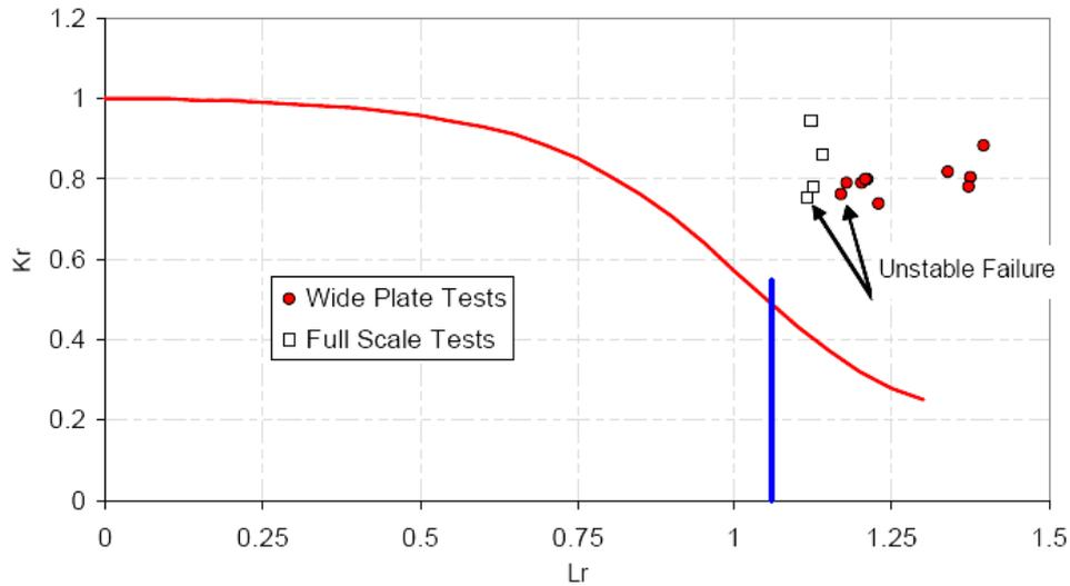
Figure 7: X100 girth weld tests from the Demopipe project [5] plotted using the BS 7910 failure assessment diagram.
