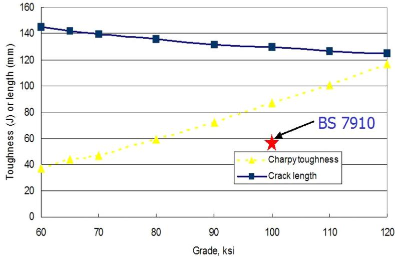
Figure 4: Critical axial through wall crack length for a 914 mm diameter 12.7 mm wall thickness pipeline operating at 80% SMYS
