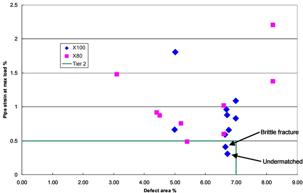
Figure 6: Curved wide plate test results for X100 [5] and X80 [15] girth welds
