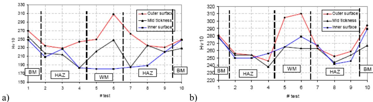
Figure 1: Typical girth weld hardness survey profiles a) SMAW 16mm WT X100 + AWS 5.5 E11018-M (WPS 4) b) GMAW 16mm WT X100 + AWS 5.28 ER100S-G (WPS 6)
