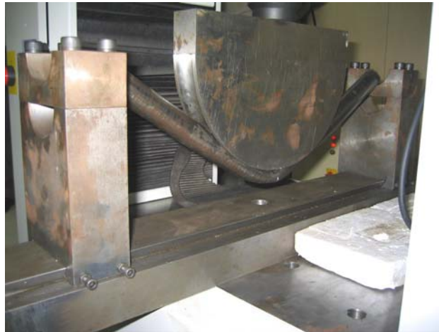
Fig.2 Bend (intrusion) test set up
