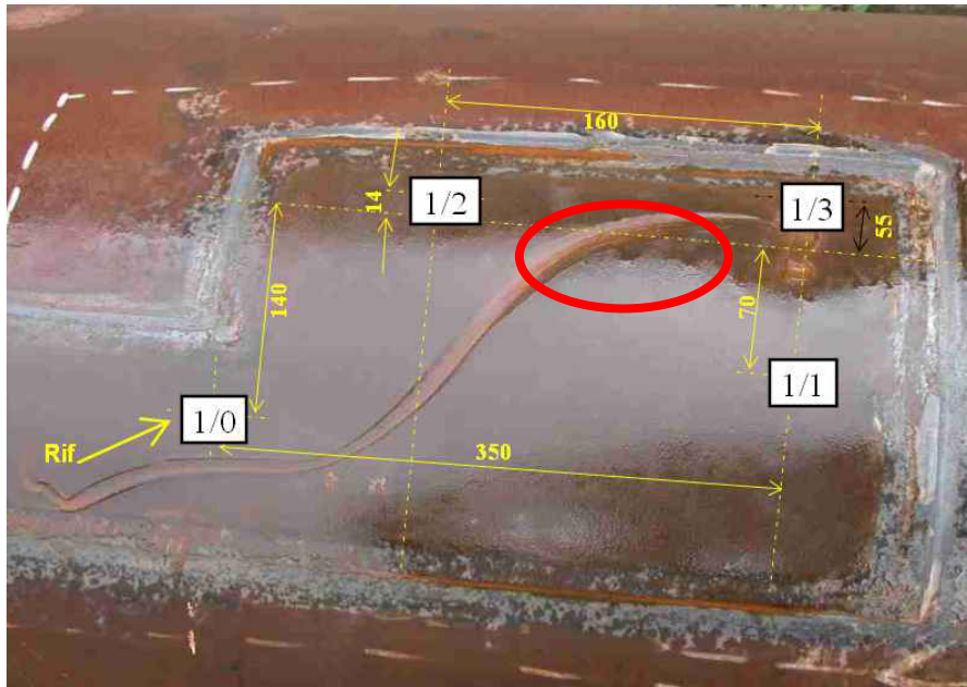
Figure 5 – Dent and gouge damage on X100 pipe with indication about strain gauges and failure location (red circle), dimension in mm.
