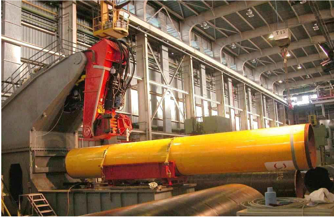
Figure 4 - CSM's full scale test aggression rig "Simulator" with a FBE coated pipe ready to be damaged (TAP project)
