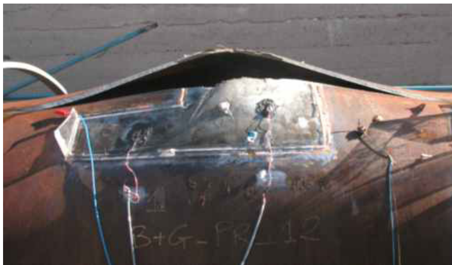
Figure 6 – View of the X100 damaged pipe after the failure
