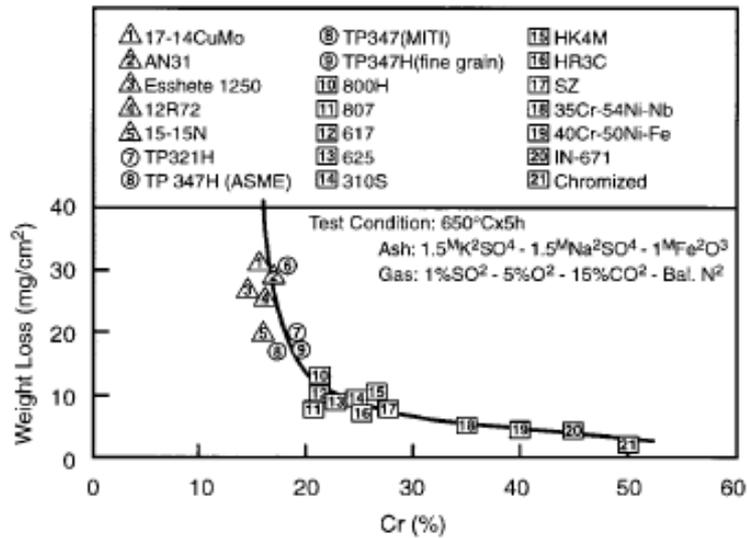
Fig. 5: Relationship between Hot-Corrosion Weight Loss and Chromium Content for Various Alloys <sup>(12)</sup>
