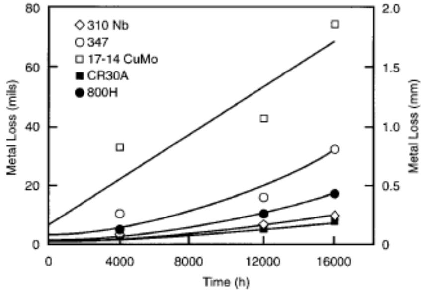
Fig. 7: Metal Losses of Various Superheater Steels in a Boiler using Bituminous Eastern US Coals<sup>[16]</sup>
