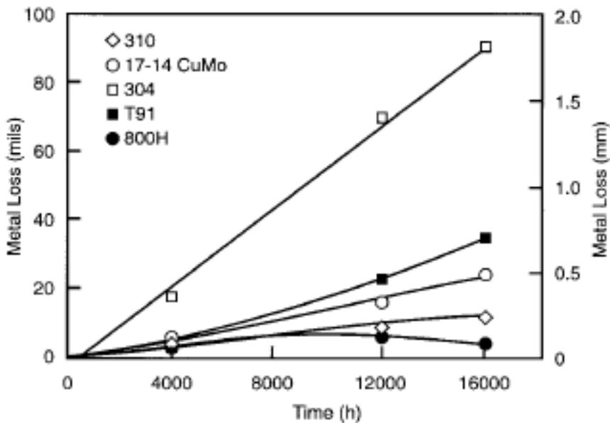
Fig. 8: Metal Losses of Various Superheater Steels in a Boiler Subbituminous Western US Coals<sup>[16]</sup>
