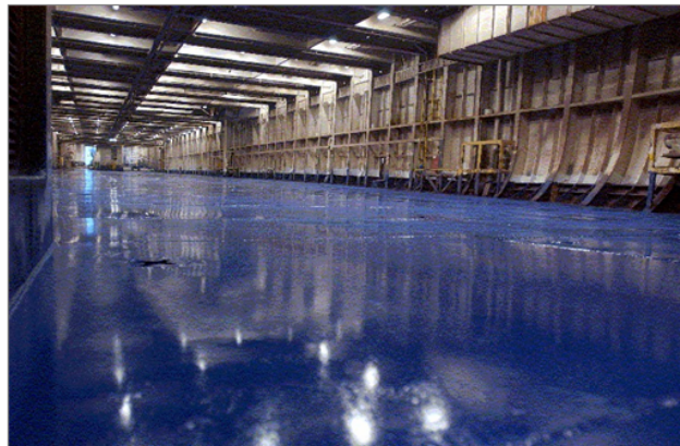
Figure 33: SPS-Overlay-techniques to refurbish the steel deck of roll-on-roll-off-ferry boats [IE-Engineering, Canada]
