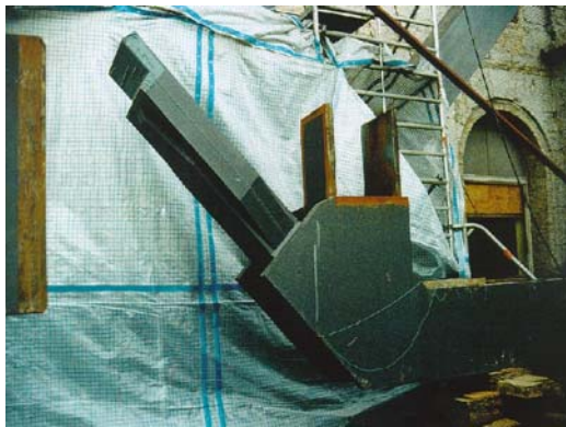
Figure 30: Details of connection of thick plates made of S460 and S690 for testing
