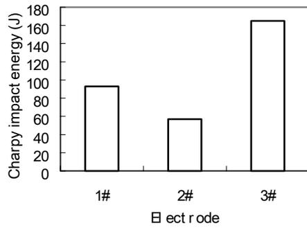
Fig.1 Charpy impact energy at -20°C
