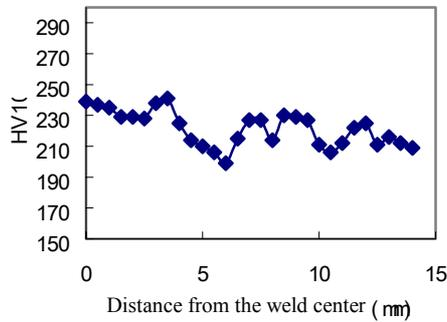
Fig.3 Hardness distribution of 2# joint
