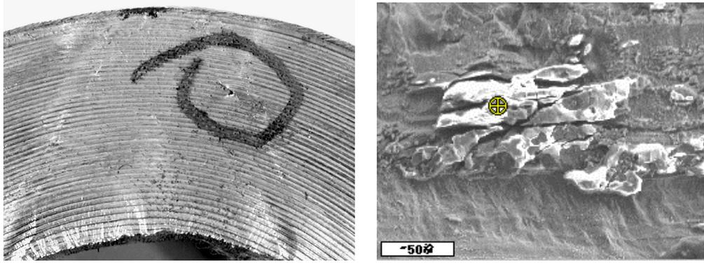
a) Defect appearance    b) Image of the internal surface of the defect
