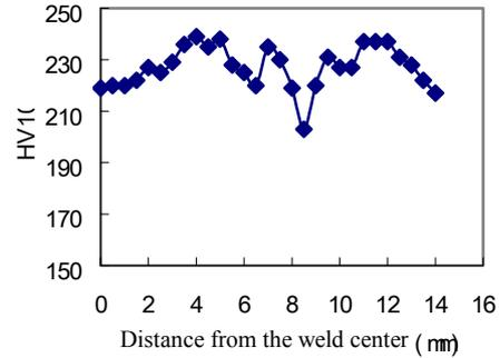
Fig.4 Hardness distribution of 3# joint
