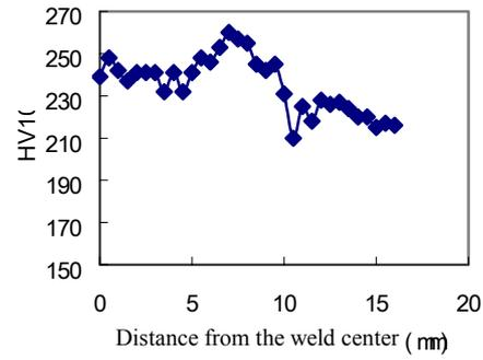
Fig.2 Hardness distribution of 1# joint
