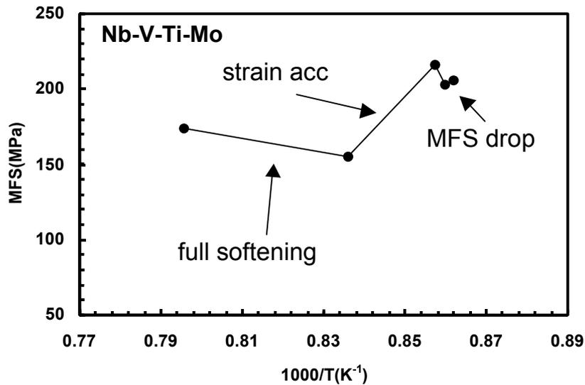
**Figure 3: Typical MFS behavior of steel Nb-V-Ti-Mo during strip rolling.**
