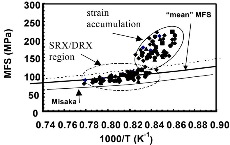
**Figure 1** Mean MFS on the high temperature side of strip rolling processing. Sims MFS was calculated from mill logs plotted vs.  $1000/T$  for several Nb containing grades, corrected to a constant strain of 0.4 and to a constant strain rate of  $5s^{-1}$  [9]. (SRX = static recrystallization; DRX = dynamic recrystallization)
