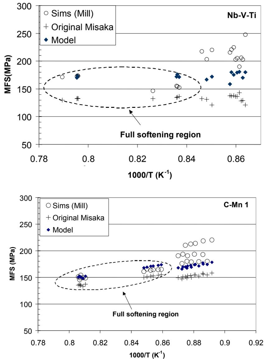
**Figure 2.** MFS vs.  $1000/T$  ( $K^{-1}$ ) charts. (a) microalloyed Nb-V-Ti and (b) C-Mn 1 grades.
