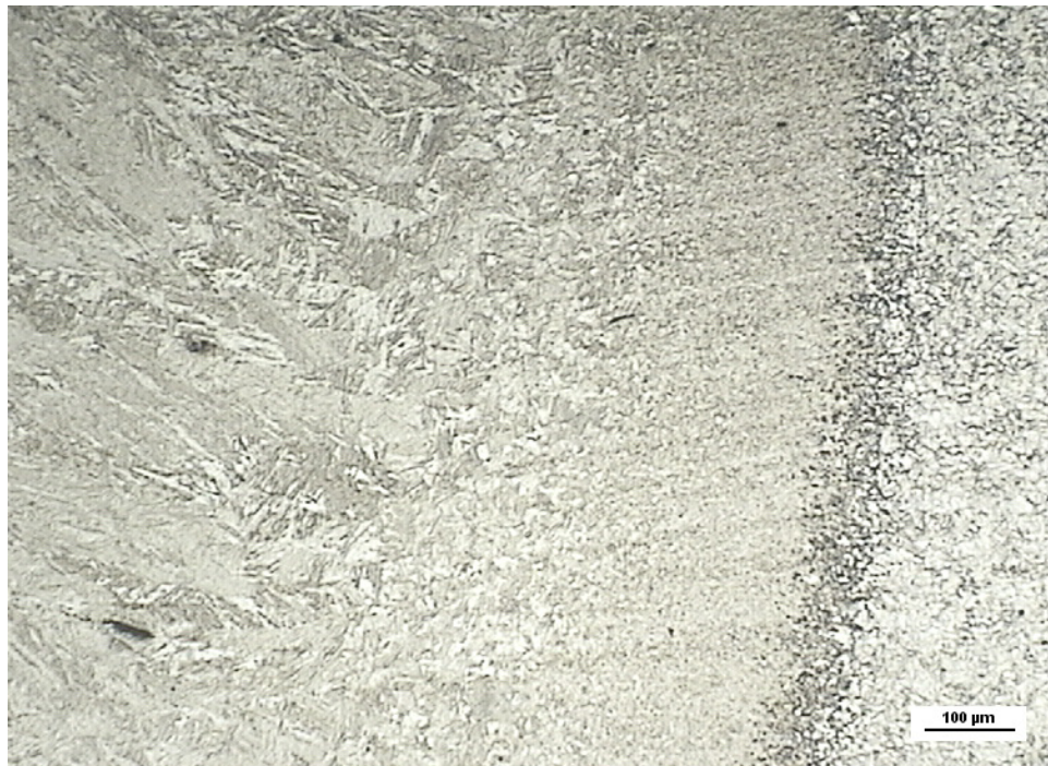
Fig.1 – Overall view of the microstructures, from left to right: fusion zone, HAZ and base metal
