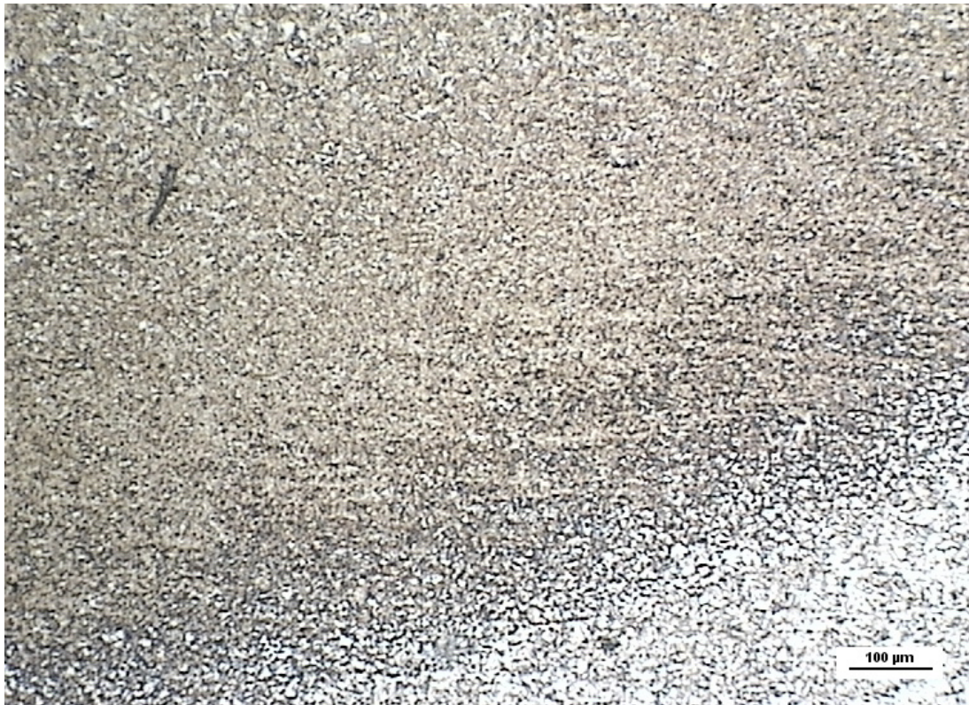
Fig.6 – SMAW joint- Overall view of microstructures. From left-high to right-low: fusion zone, HAZ and base metal
