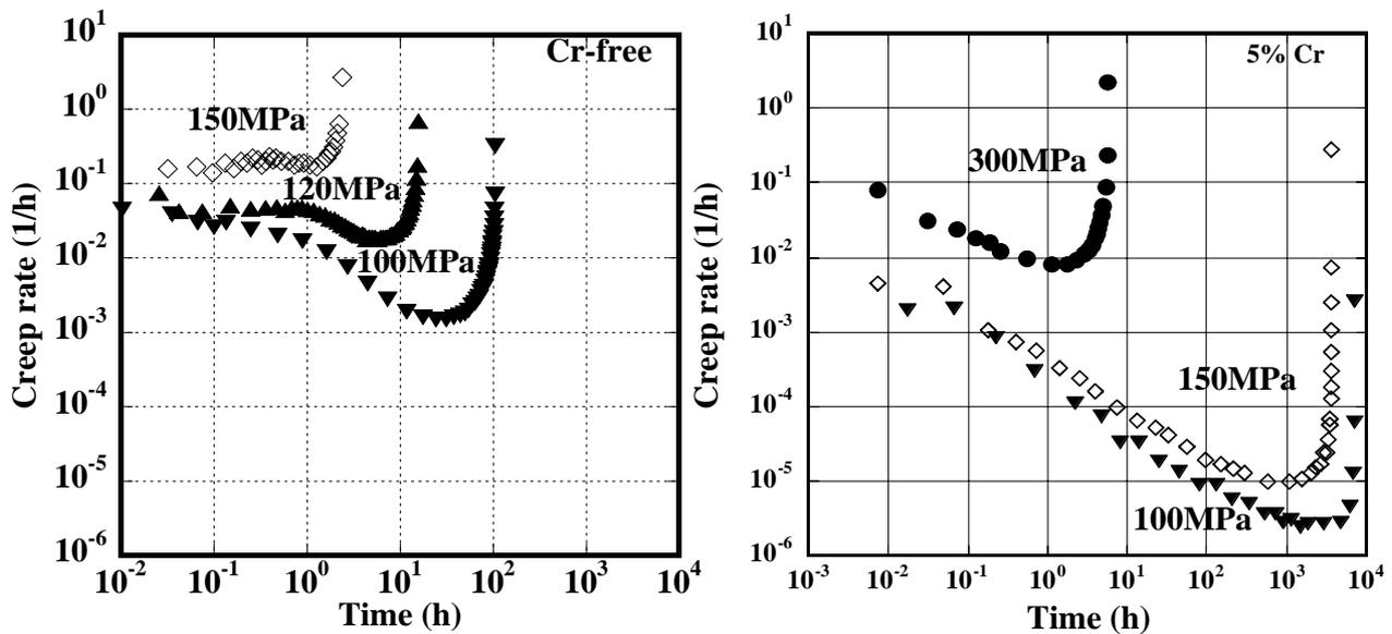
Fig.3 Creep rate vs. time curves of the Fe-12Ni-9Co-10W-0.005B alloys crept at 750 and 300 and 100MPa.
