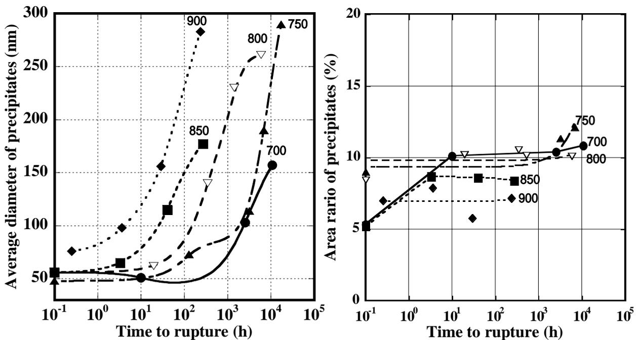
Fig.7 Changes of average diameter and area ratio of precipitates at the gage portion of the crept specimen of Fe-12Ni-9Co-10W-5Cr-0.005B alloy.
