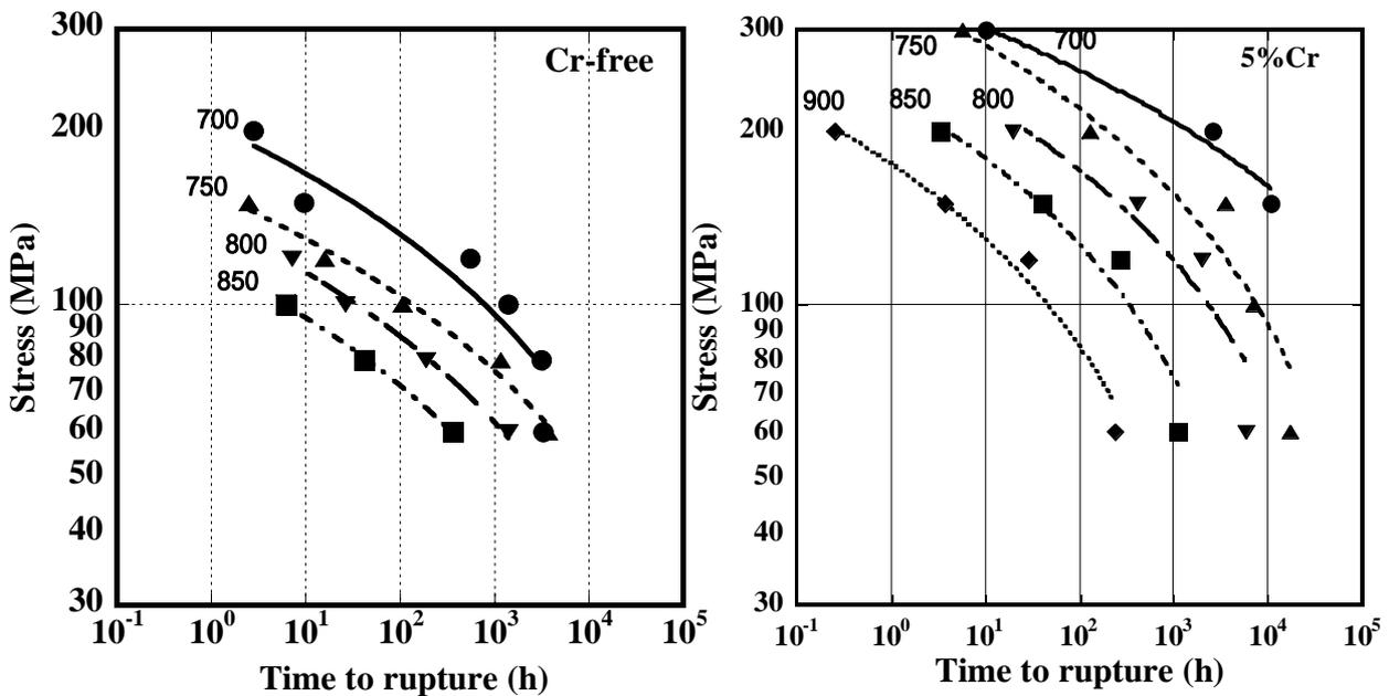
Fig. 4 Relationship between stress and time to rupture of the Fe-12Ni-9Co-10W-0.005B alloys.
