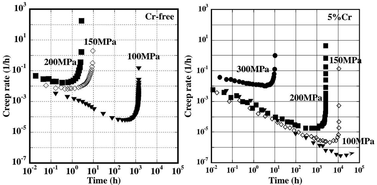
Fig.2 Effect of 5% Cr addition on the relationship between creep rate and time curves of the specimen crept at 700 in the Fe-12Ni-9Co-10W-0.005B alloys.
