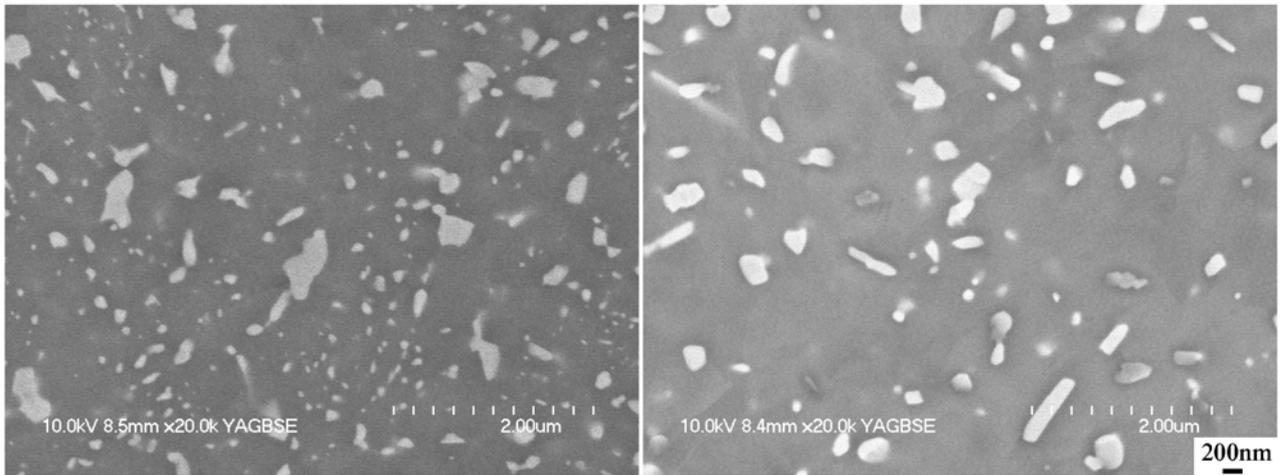
Fig.6 Backscattered electron images of the Fe-12Ni-9Co-10W-5Cr-0.005B alloy crept at a) 700°C and 2,554h and b) 800°C and 2,007h.
