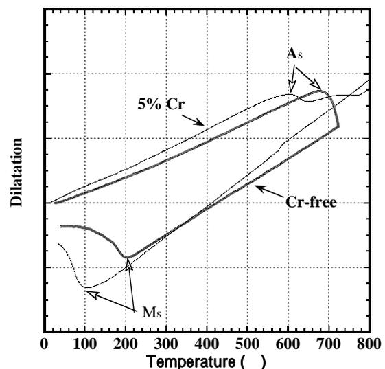
Fig.1 Effect of 5% Cr addition on the thermal expancy of the Fe-12Ni-9Co-10W-0.005B alloys.
