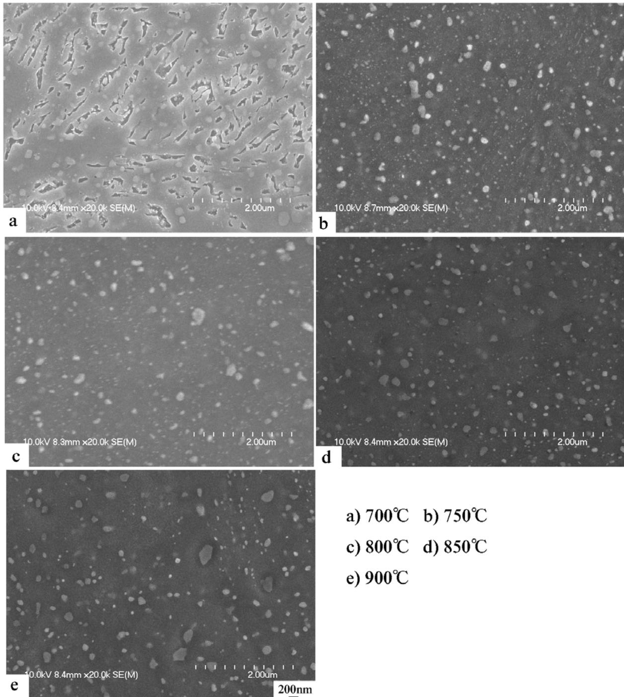
**Fig.5** Secondary electron images of the initial microstructure of the specimen crept at 700, 750, 800, 850and 900°C in the Fe-12Ni-9Co-10W-5Cr-0.005B alloy.
