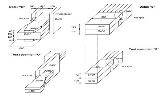
Fig. 10. Structural detailing and large scale specimens.
