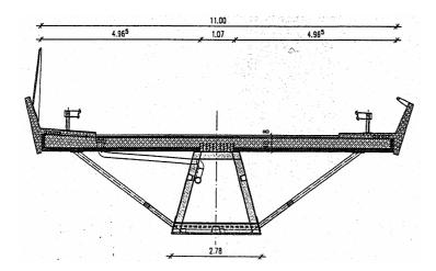
Fig. 8. Cross section of the Nesenbachtalbrücke.
