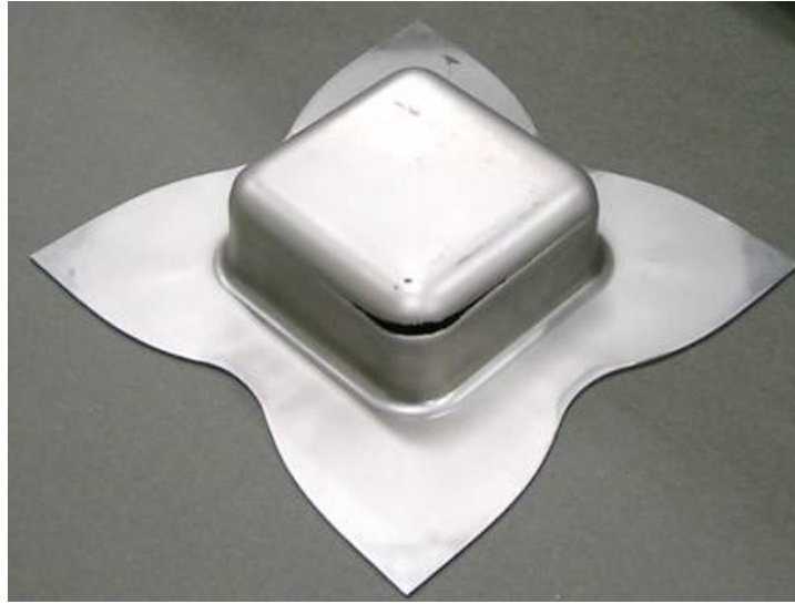
Fig. 7 Specimen after square cup deep drawing test.
