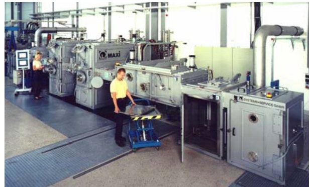
Fig. 8: In-line PVD coating plant MAXI
