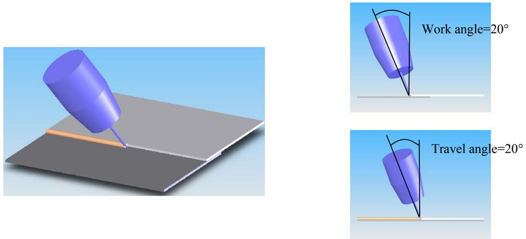
Fig. 3 : Lap joint and impact of wire for MIG process
