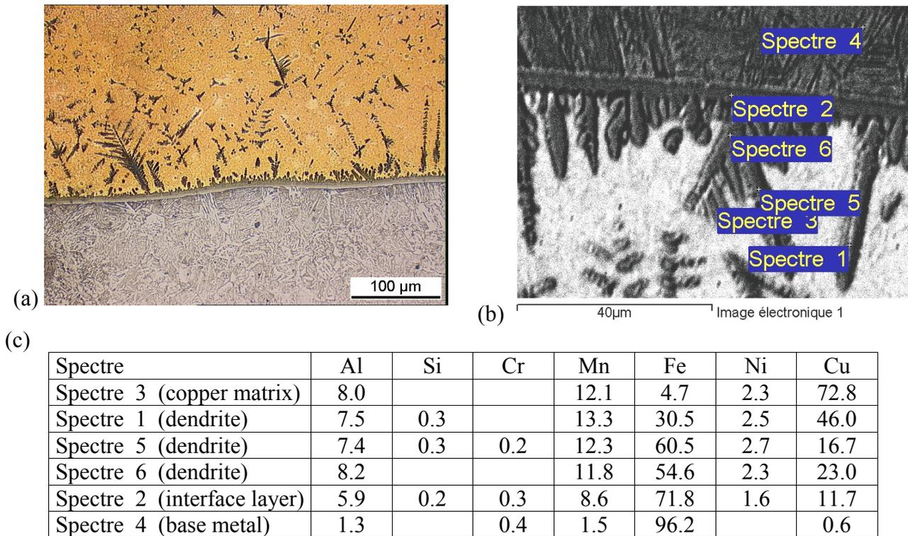
**Fig. 10 : Investigations of the interface layer for MIG weld brazing of DP600 with CuMn13Al7 filler wire (a) micrograph, (b) SEM image and (c) EDX chemical analysis of areas in (b) .**
