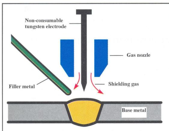
Fig. 1 : TIG process operation
