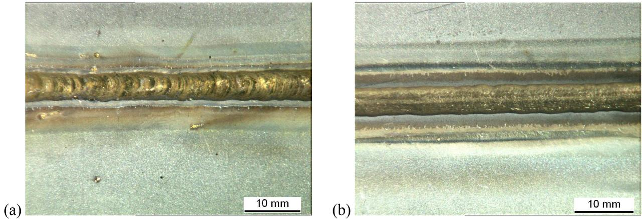
**Fig. 5 : visual aspect of beads obtained for (a) MIG braze welding on TRIP 700 with Nertalic 46 wire and (b) TIG braze welding on DP 600 with Nertalic 46 wire.**
