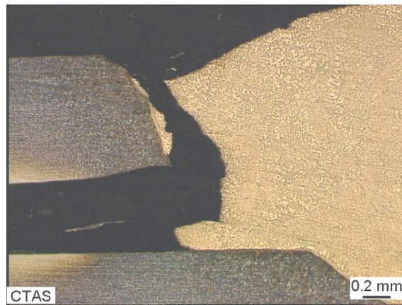
**Fig. 9 : Localization of the rupture occurring in weld metal (here on DP600 brazed with CuMn13Al7).**
