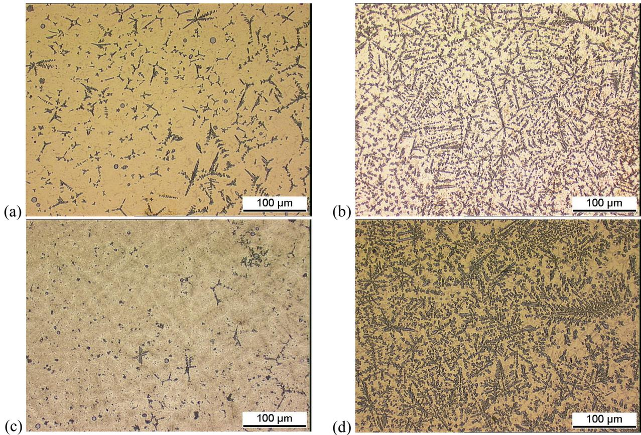
**Fig. 7 :** micrographs of MIG brazed joints obtained on DP600 with different filler wire (a) Nertalic46 CuAl8, (b) AIBz35 CuAlNi6, (c) Maxal 300 CuMn13Al7, (d) Mecufil 214Al.
