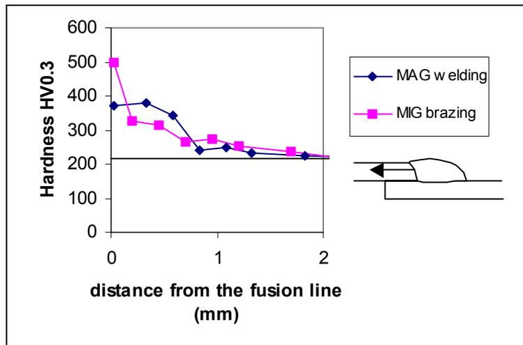
Fig. 8 : Hardness profile in Heat Affected Zone in TRIP700 steel
