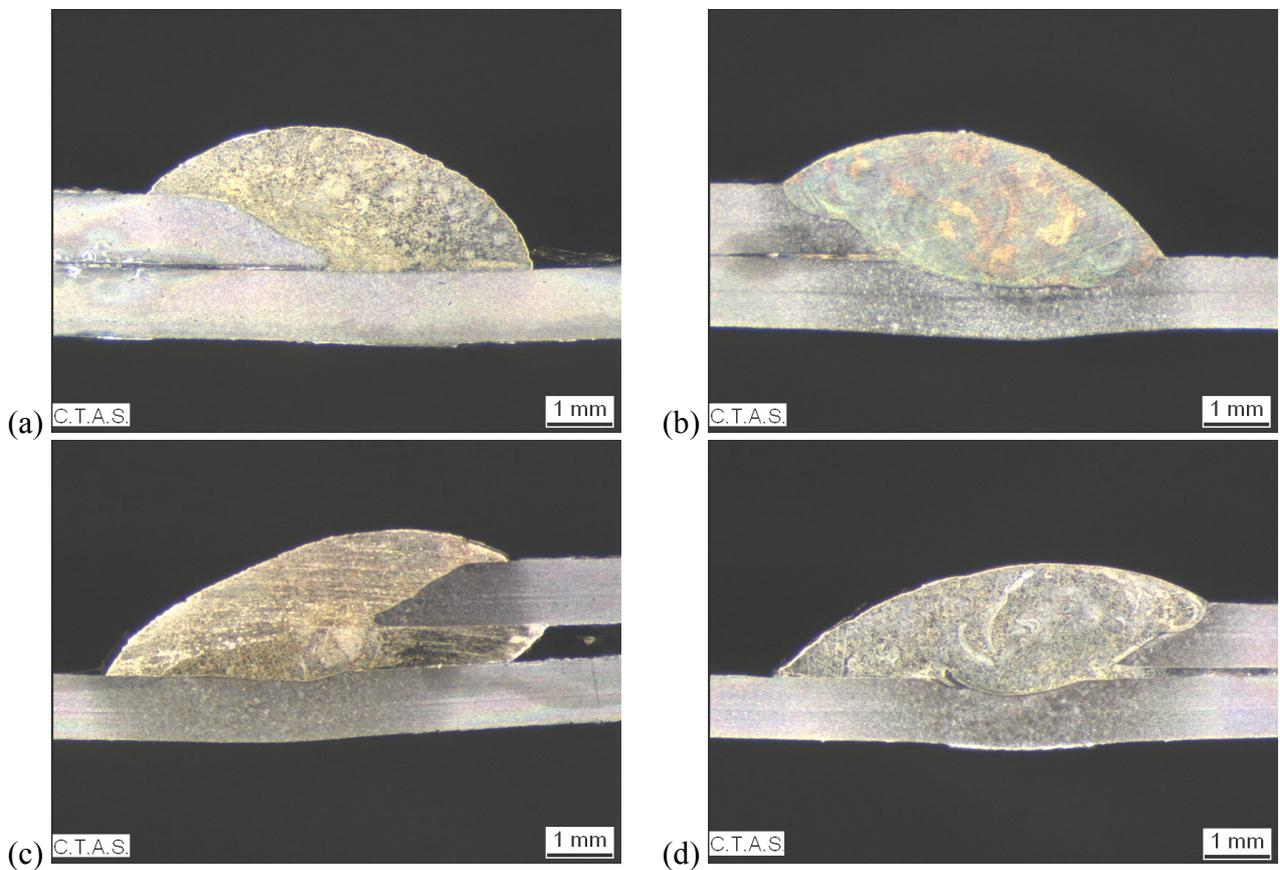
**Fig. 6 : cross sections obtained with  $\text{CuAl}_8$  wire of (a) MIG brazed joint on DP600, (b) TIG brazed joint on DP600, (c) MIG brazed joint on TRIP700, (d) TIG brazed joint on TRIP700.**
