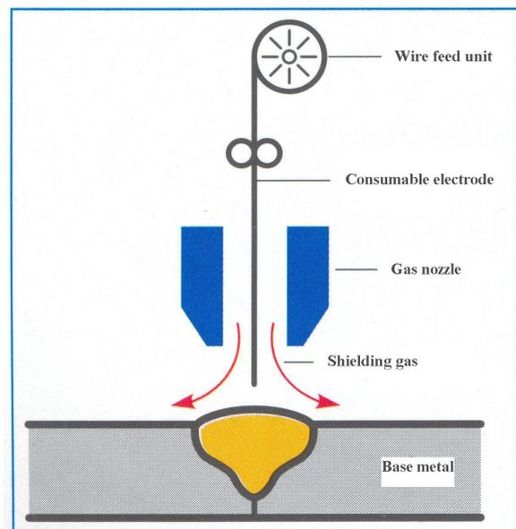
Fig. 2 : MIG process operation
