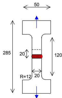
Fig. 4 : design of tensile test specimen
