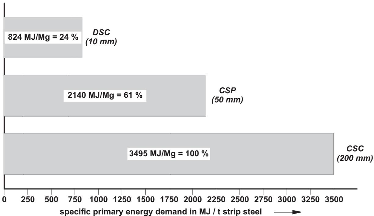
**Fig. 10:** Primary energy expenditures for CSC, CSP and DSC (casting and rolling)
