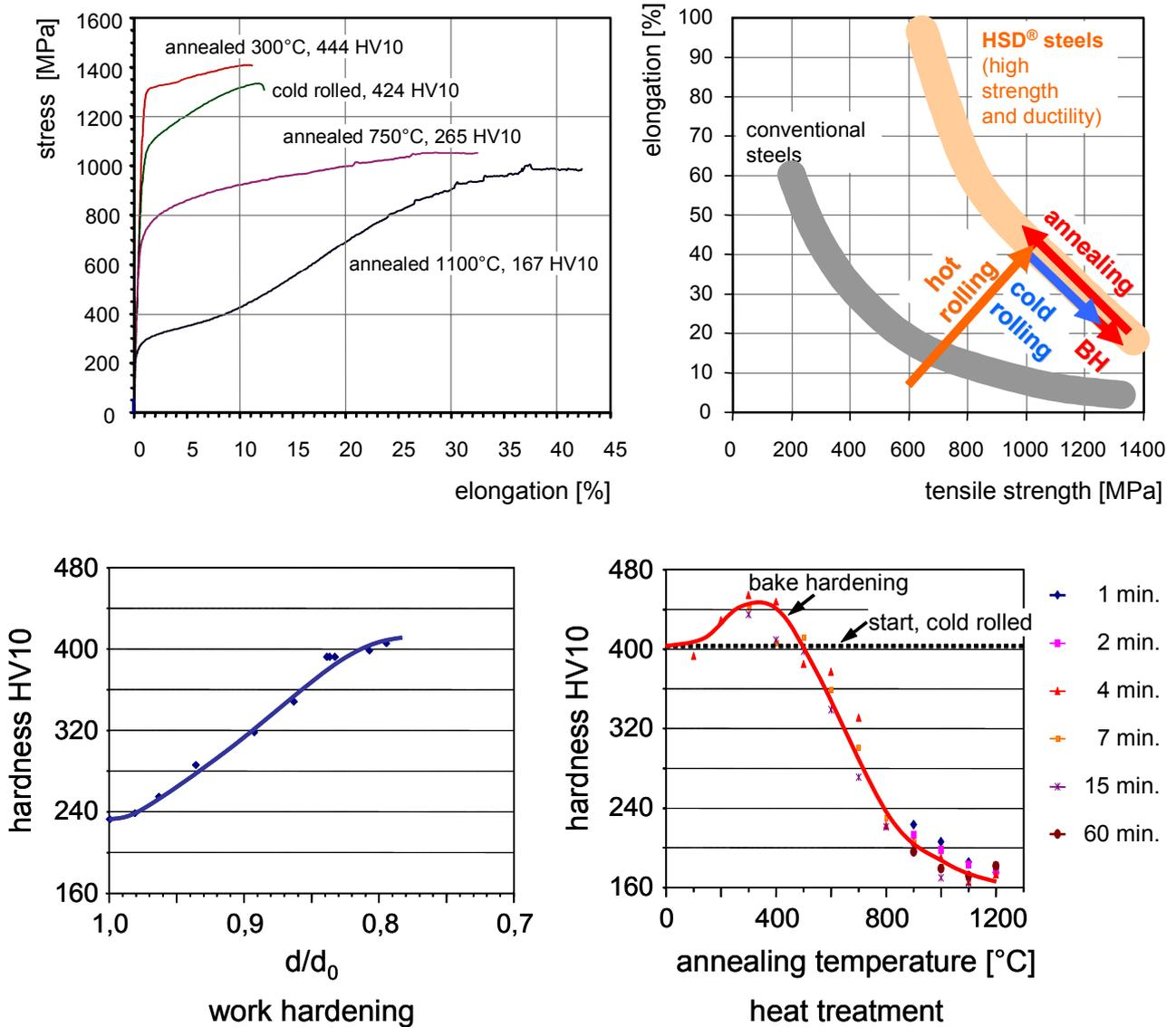
**Fig. 8:** Property adjustment by heat treatment (MnAlSi 15 2.5 2.5) at different temperatures and for different annealing times
