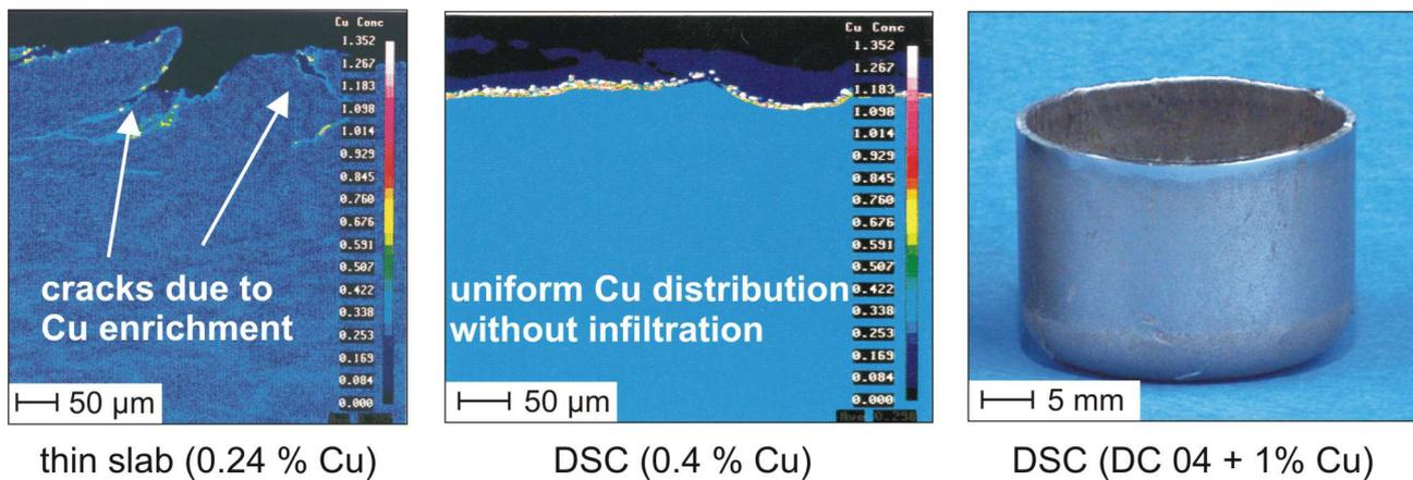
**Fig. 5:** Effects of alloying / tramp elements on surface quality
