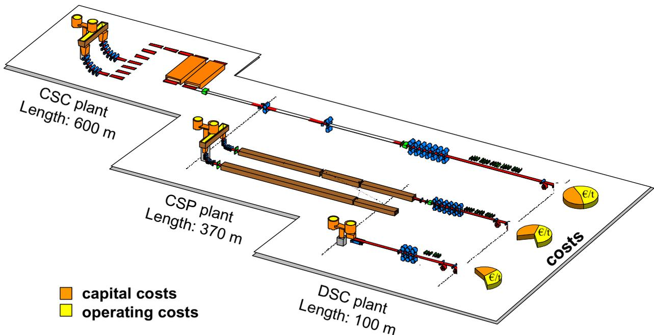
**Fig. 2:** Layout and costs of different strip production lines (for equal strip output)
