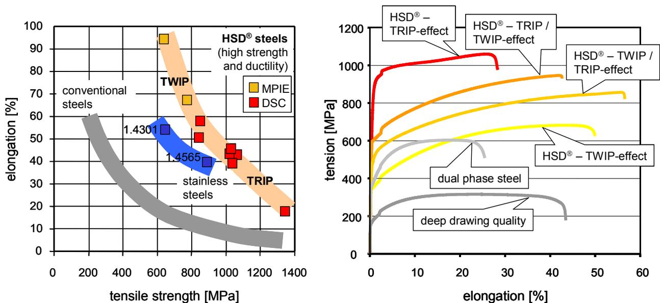
**Fig. 7:** Ductility versus strength for conventional and FeCMnAlSi HSD<sup>®</sup> steels
