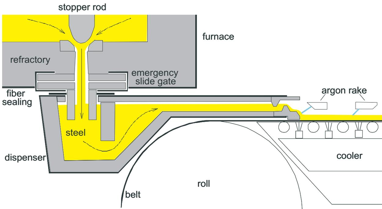
**Fig. 3:** Steel feeding system
