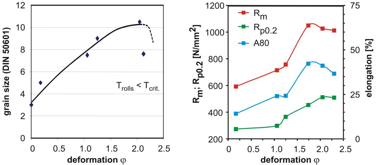
**Fig. 9:** Importance of hot rolling (MnAlSi 15 2.5 2.5); effect on structure and mechanical data
