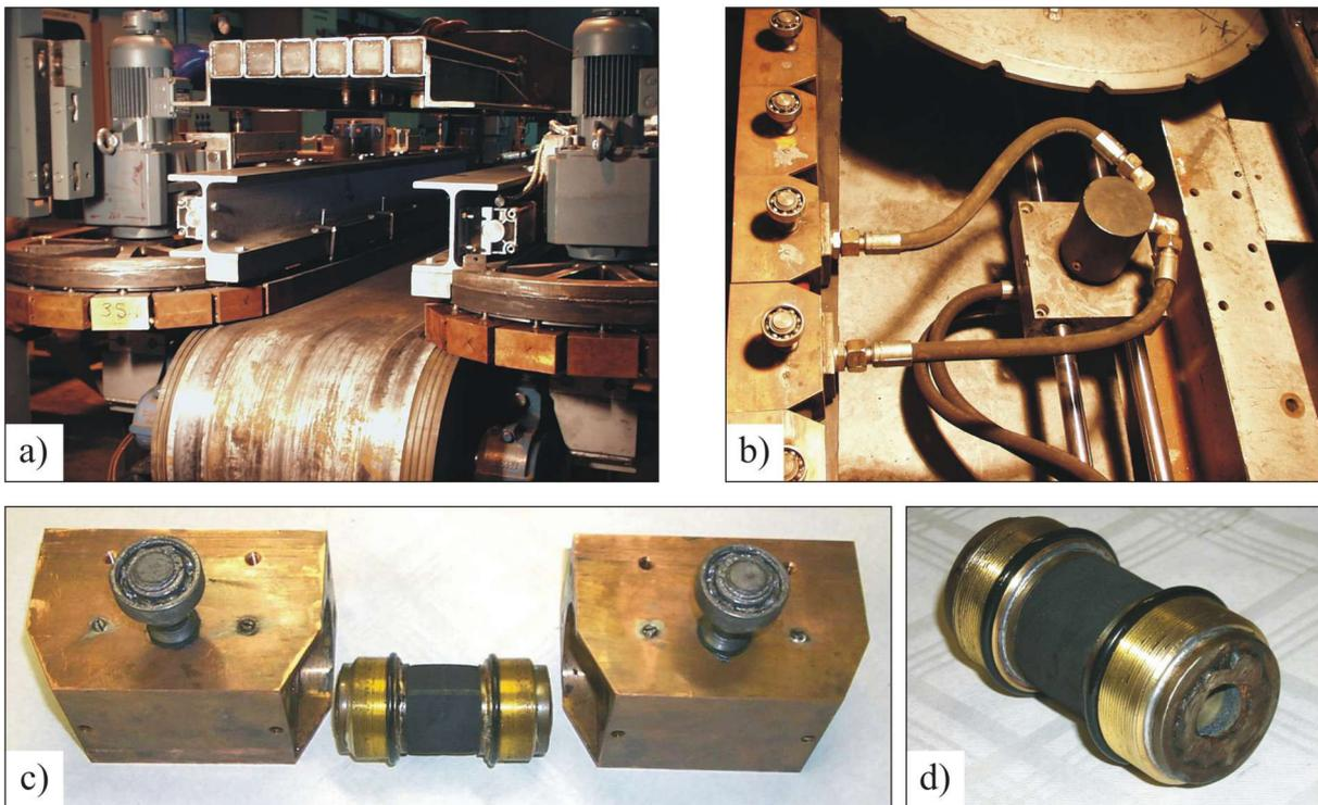
**Fig. 4:** Design of the moving side dam system
