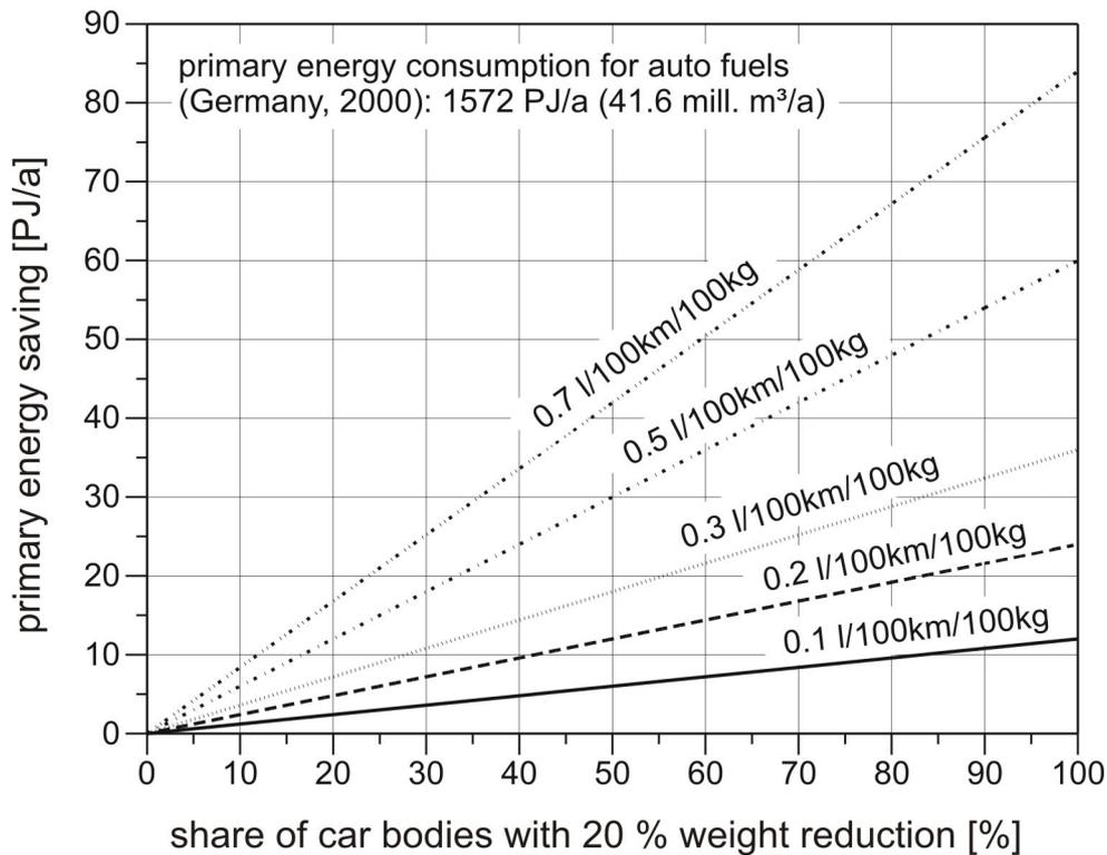
**Fig. 11:** Fuel saving potentials by FeCMnAlSi application in car body manufacturing [15]
