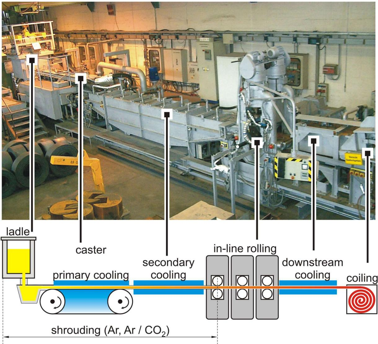
**Fig. 1:** DSC process scheme and photo of a pilot caster
