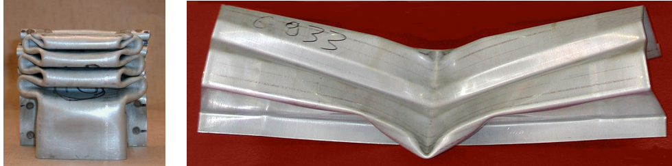
Fig. 12. Axial compression tested structure and 3-point bending tested structures after crushing
