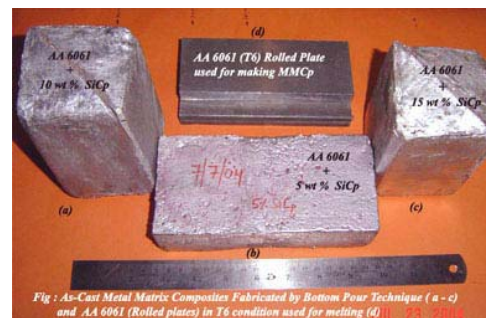
Fig 3: shows as-cast MMC in different mould shapes to facilitate testing
