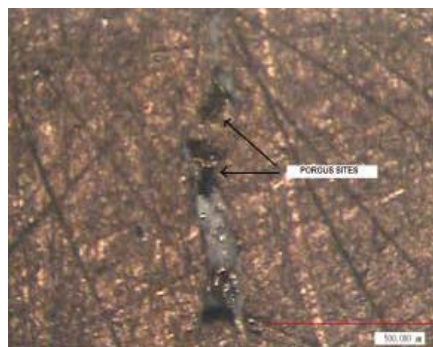
Fig. 3. Porous sites at interface of a poor joint.
