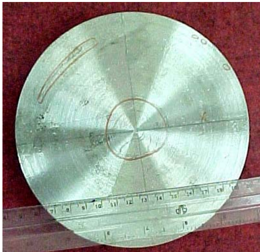
Figure 4A: Photograph of the Steel/Cupronickel sample after ultrasonic testing identifying debond locations
