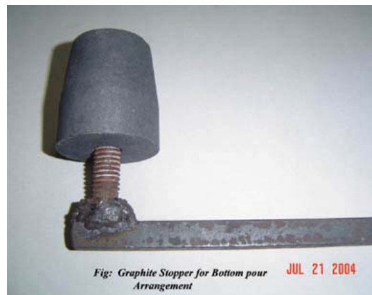
Figure. 1(a) shows the schematic of rheocasting or stircasting set up (bottom pour), (b) Graphite stopper for bottom pour arrangement.
