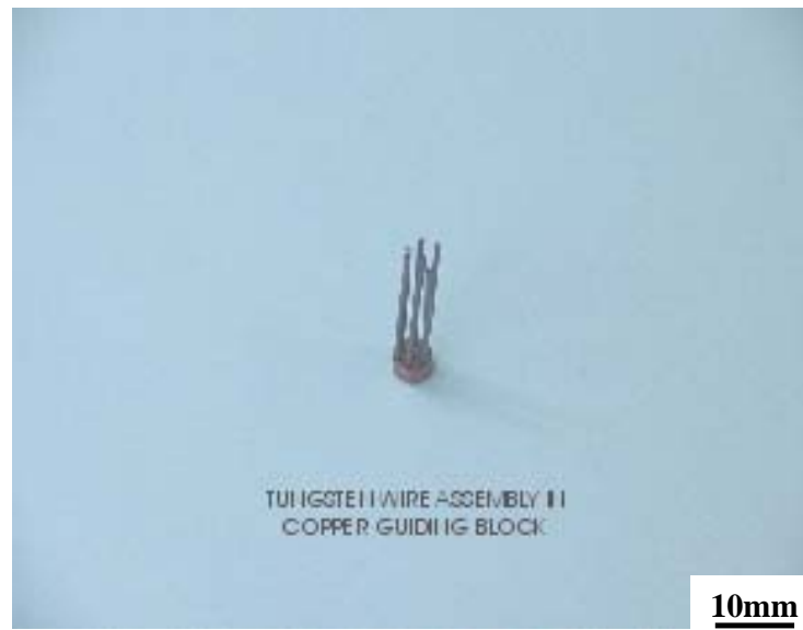
Fig. 3 Photograph showing the preform of tungsten wires.
