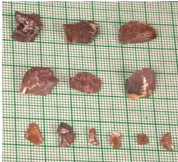
Fig.3 - Grown PZN-PT single crystal by bottom supported Bridgman method
