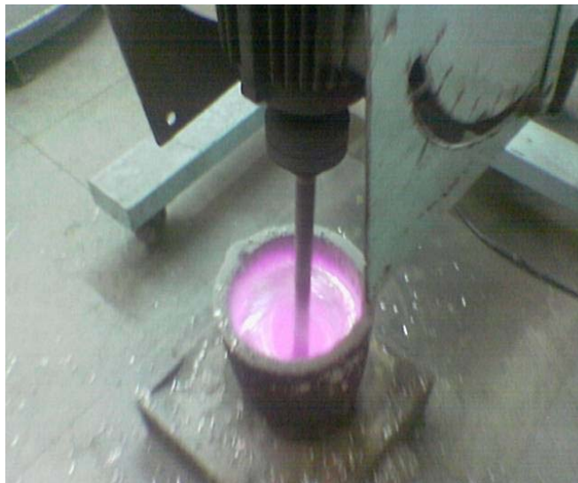
Fig (4) Mechanical Stirring of metal-particle mixture
