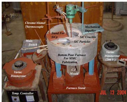
Figure. 1(a) shows the schematic of rheocasting or stircasting set up (bottom pour), (b) Graphite stopper for bottom pour arrangement.
