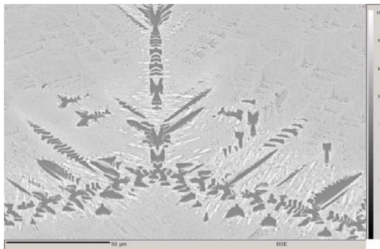
Fig. 5(b) Back scattered electron image of the arc melted microstructure of the glass forming alloy.
