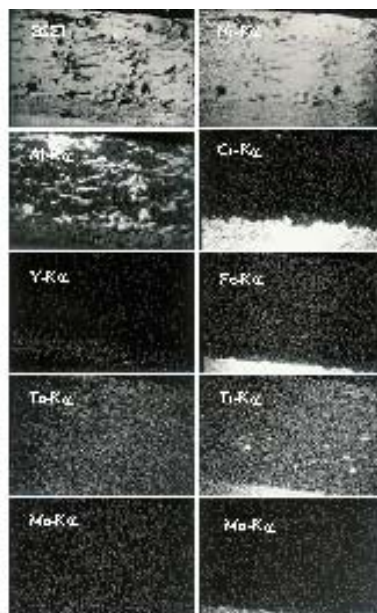
Fig9 BSEI and elemental Xray mapping of the cross-section of plasma sprayed NiAl coating with bond coat of NiCrAlY on superalloy 718 superalloy.
