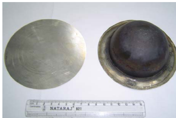
Fig. 7 superplastically bulge-formed component (right) and the blank before forming (left).
