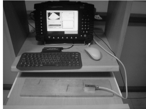
(b) Experimental setup of Phased Omniscan MX with a 5 MHz
