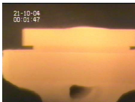
Fig 5. Still image of liquid silicon droplet on graphite substrate (a) droplet 1 s after melting (b) after 23 s c) after 60 s.
