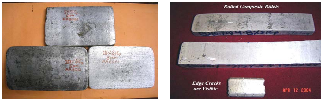
Fig 4: As-cast Composite Rolled Billets
