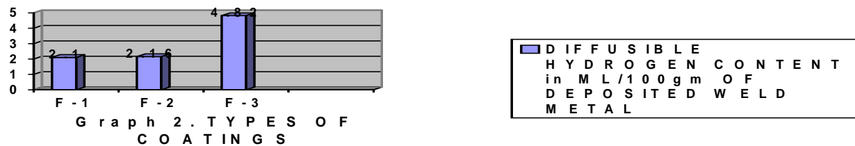
VARIATION IN DIFFUSIBLE HYDROGEN CONTENT OF WELD METAL WITH VARIATION IN COATINGS
