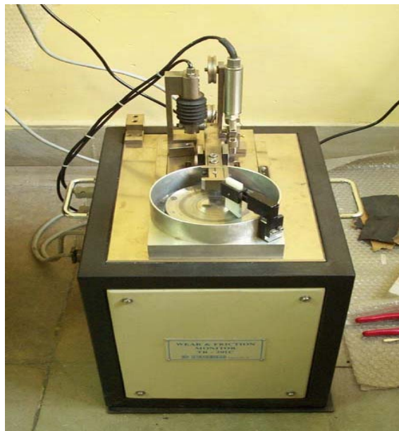
Fig (6) Computerized pin on disc wear testing machine
