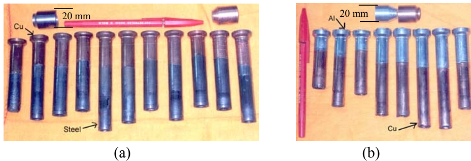
Fig. 7 Successful transition joints made by cold extrusion of P/M preforms (a) steel-Cu (b) Cu-Al.
