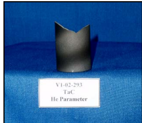
Fig. 6: Vacuum Plasma Sprayed Near Net TaC Cylinder
