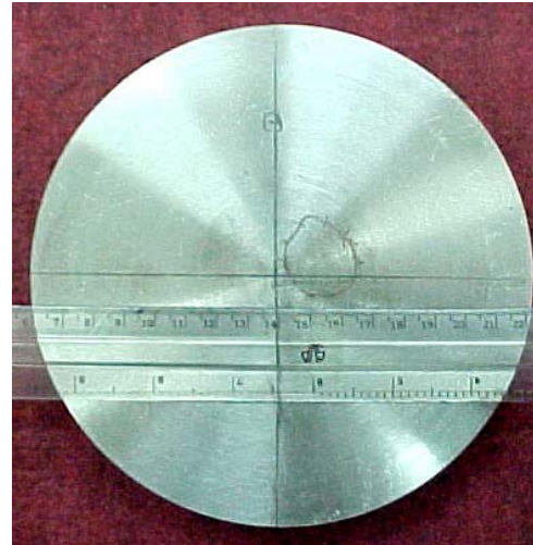
Figure 4B: Photograph of the Steel/Titanium sample after ultrasonic testing identifying debond locations
