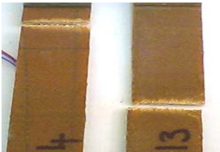
Figure 4. Typical tensile failure modes
