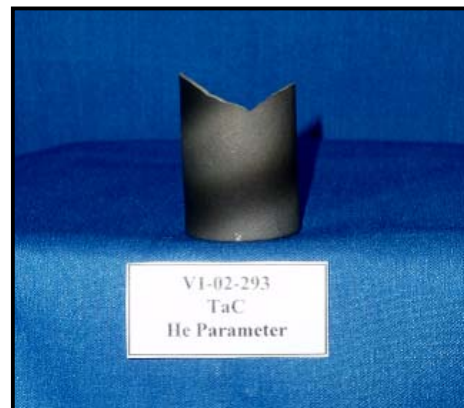
Fig. 6: Vacuum Plasma Sprayed Near Net TaC Cylinder
