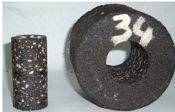
Figure 2 Triaxial test specimen cored from Marshall Sample
