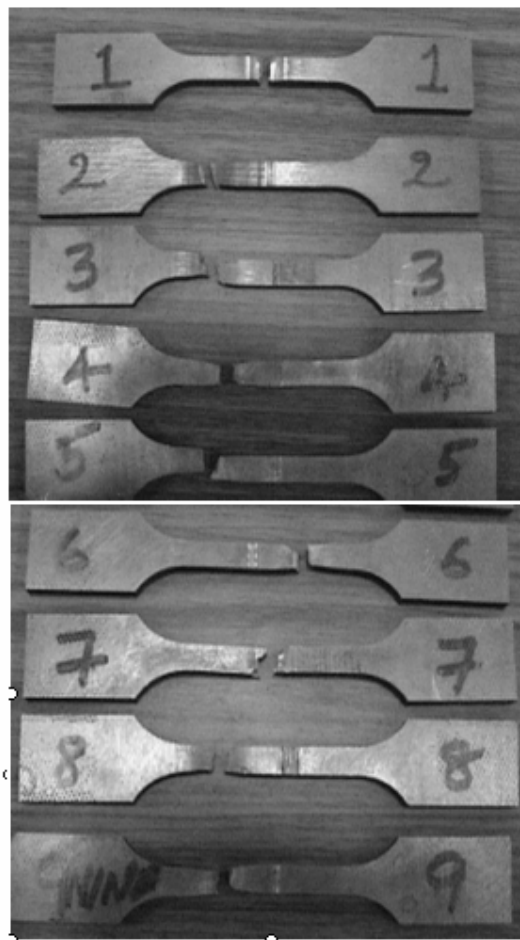
Fig 7. Tensile test specimens after Testing
