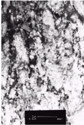
Fig. 1 Initial microstructure of N+T Modified 9 Cr-1 Mo ferritic steel
