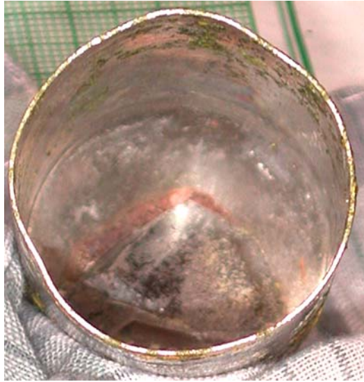
Fig.2 - Grown PZN-PT single crystal with platinum crucible
