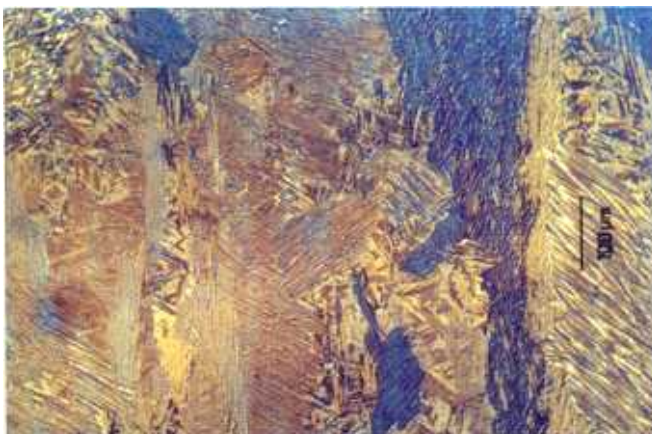
Figure 7. Typical microstructure of an all-weld metal deposited with the supermartensitic metal-cored wire OK Tubrod 15.55 (<0.01%C, 12%Cr, 6.5%Ni, 2.5%Mo).
