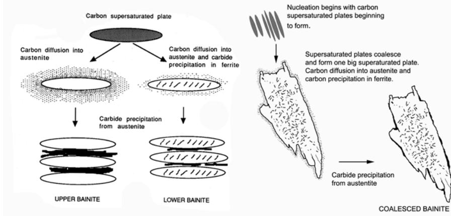
Figure 4: Schematic representation of the formation of upper and lower bainite [12] along with coalesced bainite [11].
