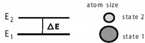
Figure 3: A schematic representation of the two atomic states in the two-state invar model. The higher energy state having a lower atomic volume (image from Lawson et al , 2003)
