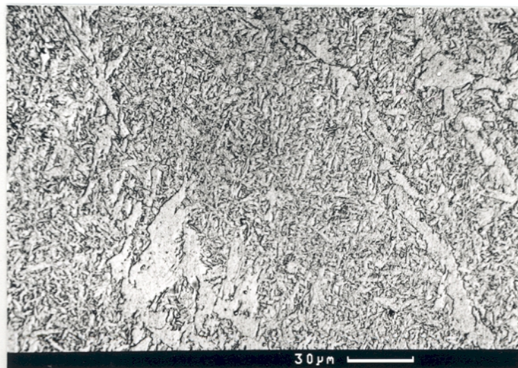
Figure 3 SEM micrograph of the as-deposited microstructure in Weld B.
