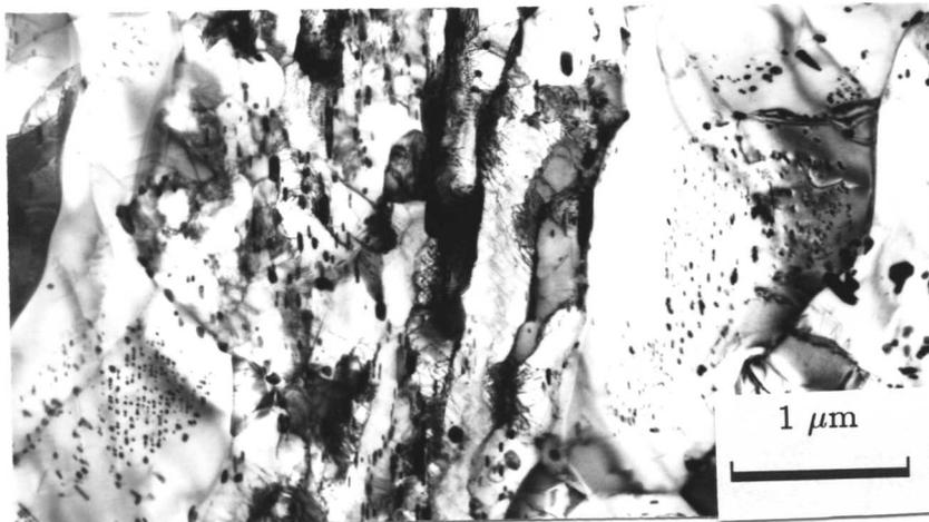
Fig. 5.14: *Recrystallised microstructure observed in specimen after 31 days of tempering at 600 °C, TEM thin foil micrographs.*
