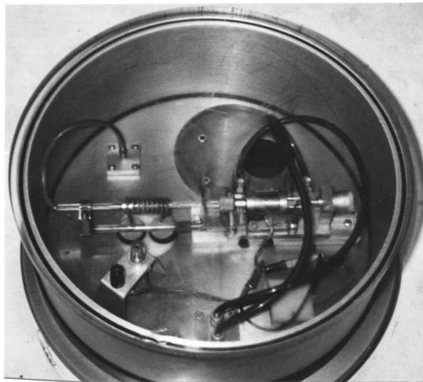
Fig. 3.2: Photograph showing the dilatometer and its test chamber, as used in this study.
